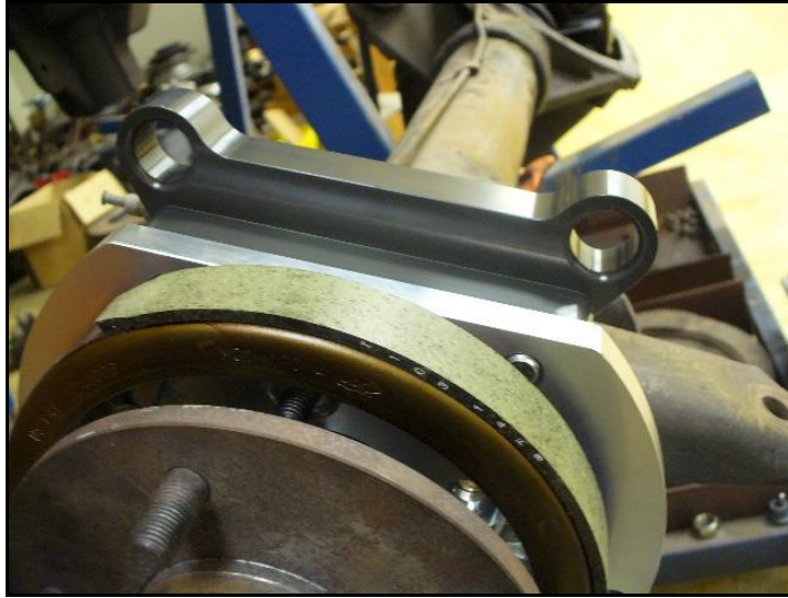
Figure 3: Park brake assembly correctly installed
