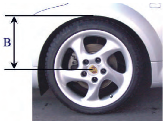
Measurement B Wheel hub center wheel arch
