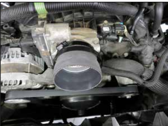
20. Install the 08497 hose to the throttle body with clamps provided for 5.3L models. Install the 084107 hose for the 6.2L models. Tighten clamps using 5/16" socket or nut driver. Note: Do not over tighten clamps.
