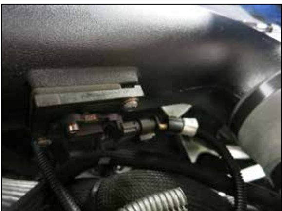
24. Connect the MAF sensor using provided harness extension, and secure harness using cable tie.
