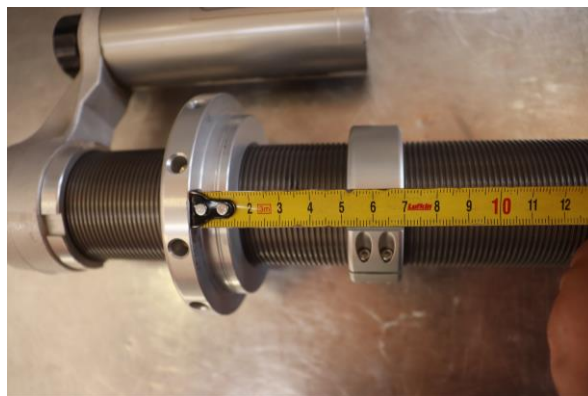
Step 12. Install Eibach crossover ring and adjust to 70mm (2 3/4 in) .
