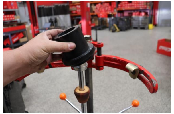
Step 14. Install Eibach front spring slider with the short end facing the top of the shock.
