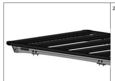
20. With assistance, carefully place the BASE RACK on the vehicle so the inside of the blade brackets rests on the outside of the mounting brackets. The entire BASE RACK assembly should be clear of the vehicle roof. All mounting holes/slots should align closely.
