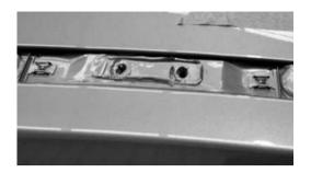
1. Remove 2x LH and 2x RH plastic covers shown from each gutter.
