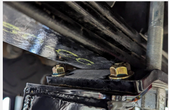
Figure 7: Relocation Brackets tight
