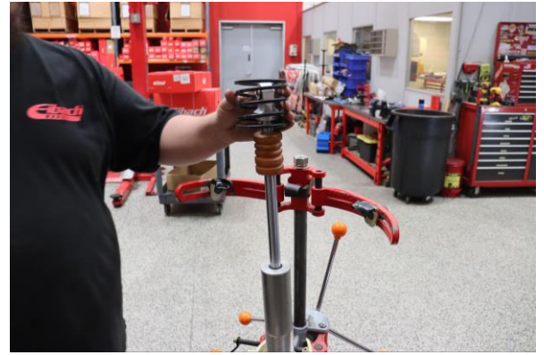
Step 14. Remove the second OE tender spring.
