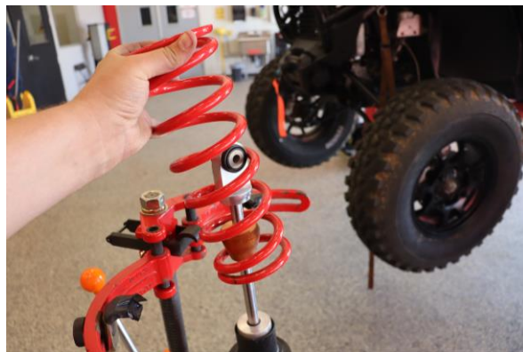
Step 8. Remove the OE main spring.
