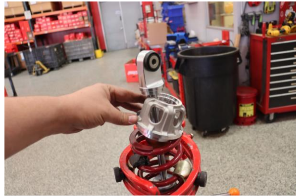
Step 16. Install OE lower spring perch. Decompress assembly and ensure lower spring perch engages lower shock mount fully.
