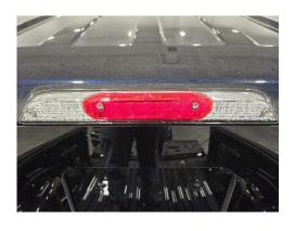
3. Remove the 3rd brake light by pulling outwards from the bottom of the light and unplugging the 3rd brake light from its harness.
