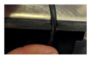
6. Peel off the 3M tape backing on the front of the bracket, feed the wires through the bracket and reconnect to the 3<sup>rd</sup> brake light.
