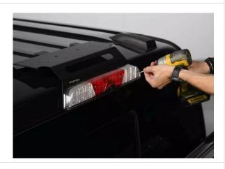
8. At this point, install the hornet light on to the mounting bracket using the 10-32 nuts and bolts. This will require the 1/8" Allen and the 3/8" wrench. You can fish the wire through the hole in the bracket for a cleaner look.
