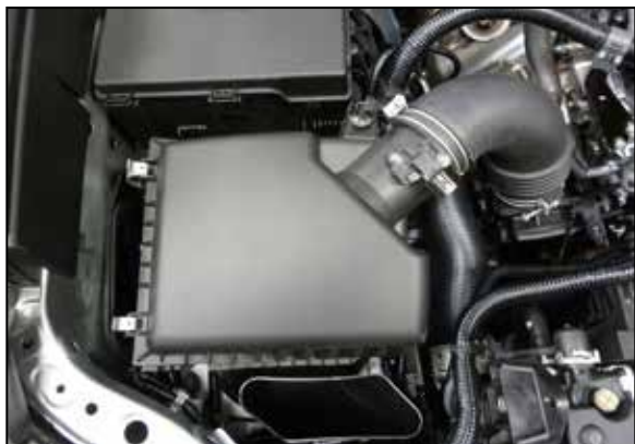
5. Lift the complete intake system straight up and remove it from the vehicle. NOTE: K&N Engineering, Inc., recommends that customers do not discard factory air intake.
