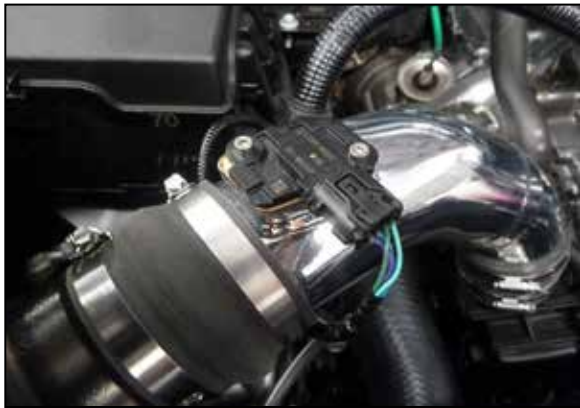
15. Connect the mass air sensor electrical connection.
