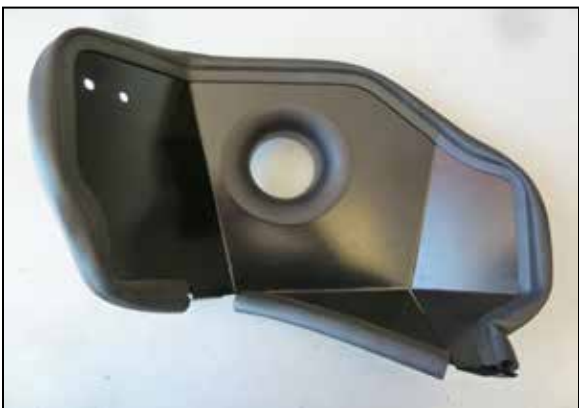
8. Install the filter adapter into the heat shield and secure with the provided hardware.
