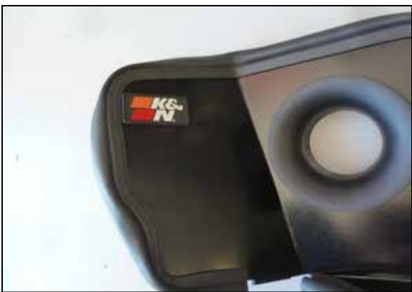
9. Install the K&N badge into the heatshield and secure with the backing plate.
