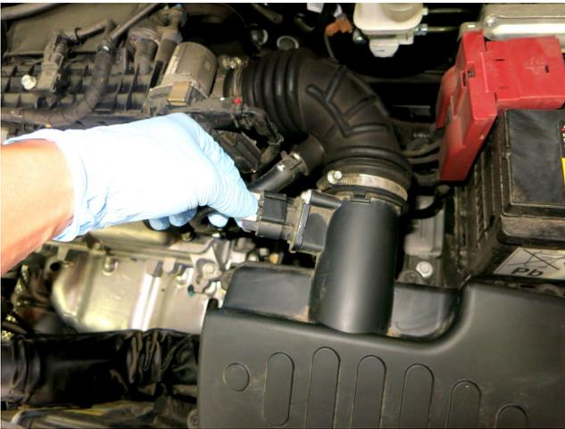
a. Disconnect the mass air sensor connector by sliding the gray locking tab and depressing the tab.
