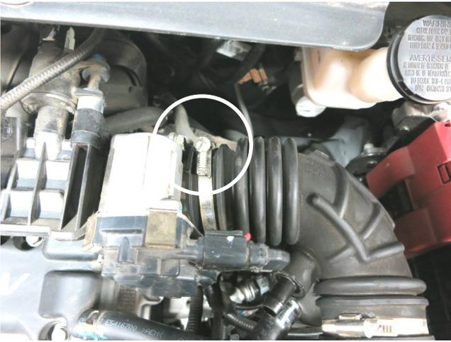
e. Loosen the hose clamp at the throttle body and disconnect the stock intake from the throttle body.
