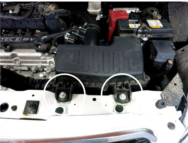
c. Remove the two bolts holding the front of the stock air box to the vehicle. One of these will be reused in step 3f.
