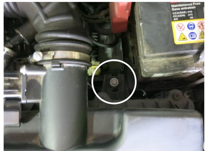
d. Remove the single bolt holding the rear of the stock air box to the vehicle.
