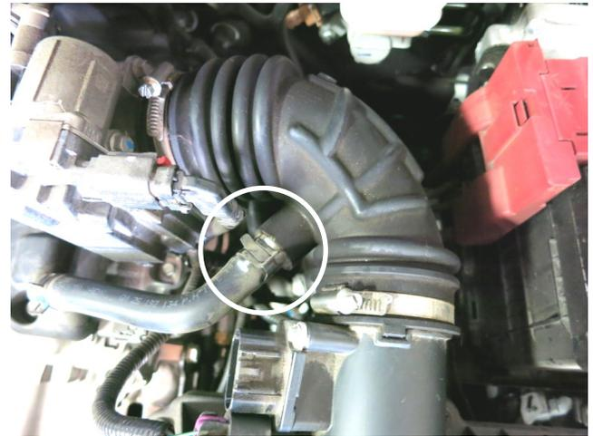
b. Loosen the spring clamp and remove the vent tube from the stock intake tube. The spring clamp will be reused in step 3k.
