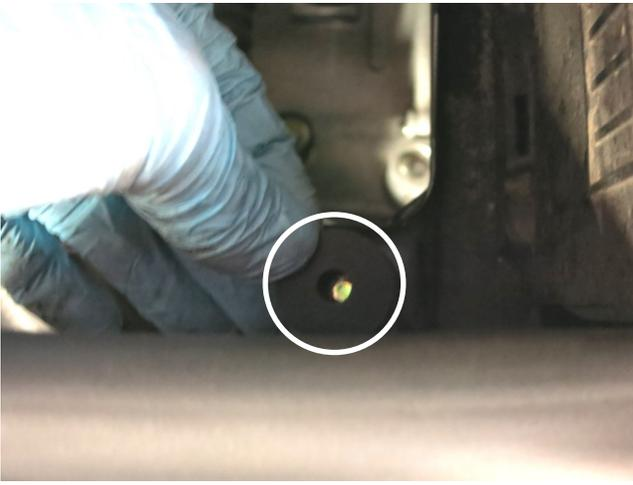
g. Align the heat shield with the rubber mounted stud that was previously installed and place the provided rubber washer over the stud.
