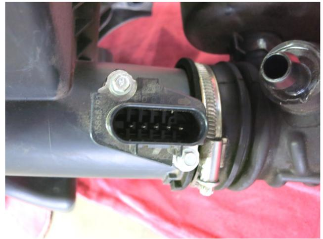
h. Remove the two bolts securing the Mass Air Flow sensor from the stock intake. The sensor will be reinstalled in step 3a. **NOTE: DO NOT DISCARD ANY OF YOUR STOCK EQUIPMENT.**
