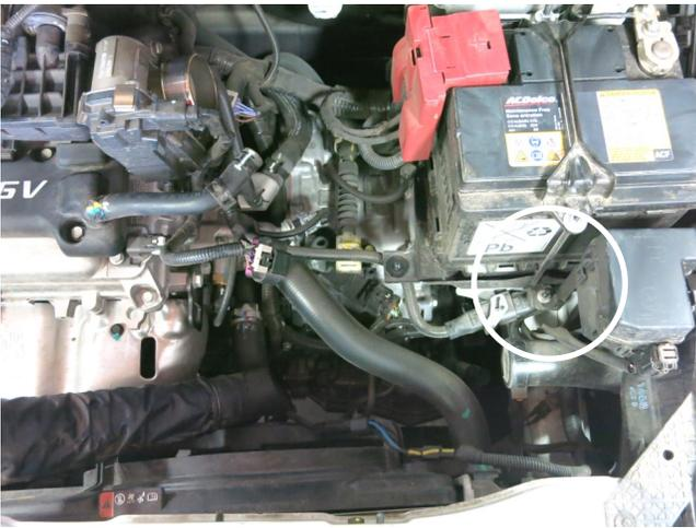
g. Remove the M6 nut in front of the battery as circled. This nut will be reused in step 3h.
