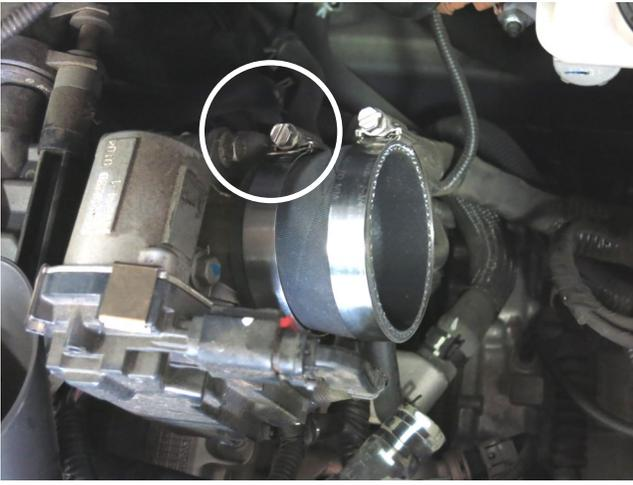
i. Install the provided coupler and hose clamps onto the throttle body. Tighten the hose clamp circled at this time.
