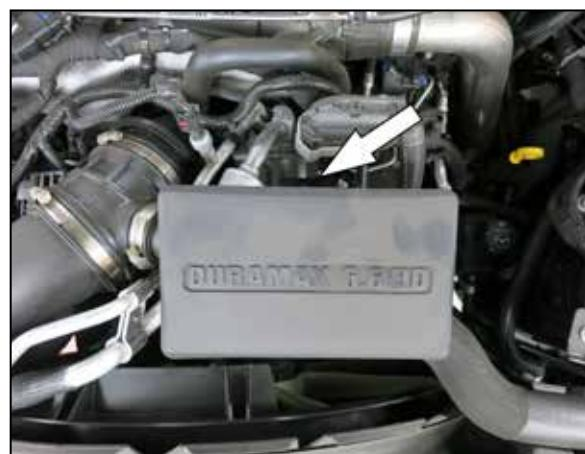
3. Remove the nut that secures the intake plenum to the engine.
