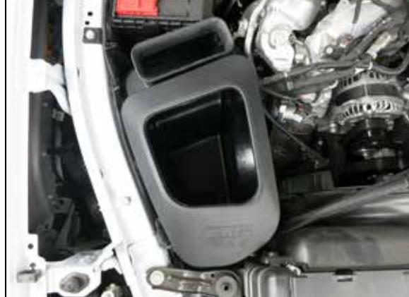
9. Install the K&N air filter housing into the vehicle and secure with the factory mounting nut.
