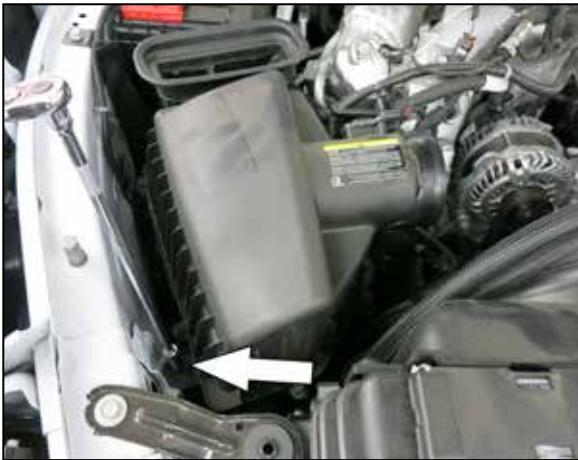
5. Remove the nut that secures the factory air filter housing to the inner fender, then remove the housing from the vehicle. This nut will be reused. **NOTE: K&N Engineering, Inc., recommends that customers do not discard factory air intake.**
