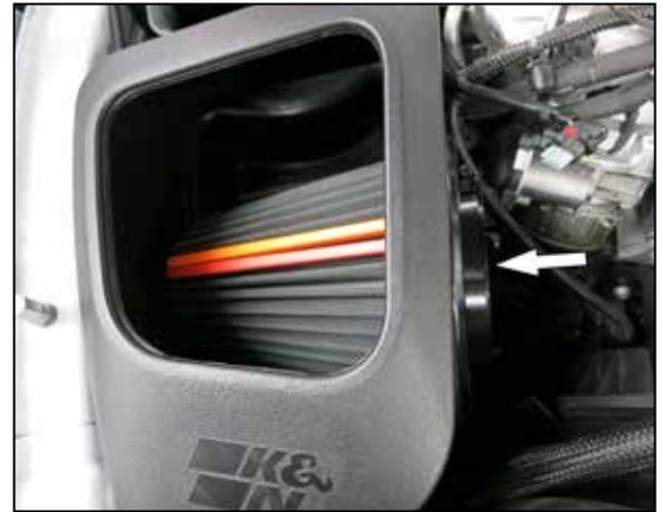
11. Install the K&N air filter into the housing as shown.
