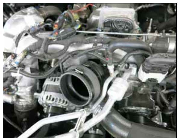
12. Install provided hump coupler onto the turbo inlet with the provided hose clamps.
