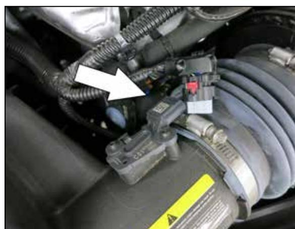
2. Release the locking tab and then disconnect the mass air sensor electrical connection.
