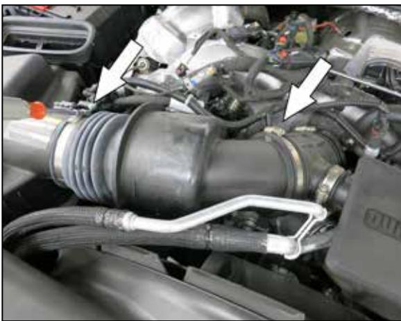
4. Loosen the hose clamps that secure the intake tube to the turbo inlet and the air filter housing outlet, then remove the factory intake tube assembly from the vehicle.
