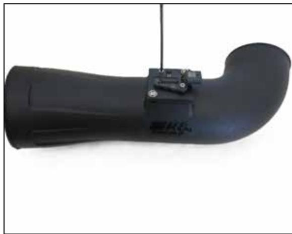
7. Install the MAF sensor assembly into the intake tube and secure using provided hardware. Secure and tighten. **NOTE: Make sure the sensor is going in the correct direction.** If it is not installed in the correct orientation, remove the adapter bolts and spin 180 degrees then reinstall the bolts.
