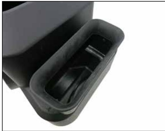
8. Install the fresh air inlet seal onto the K&N air filter housing and secure with the provided retaining clips.
