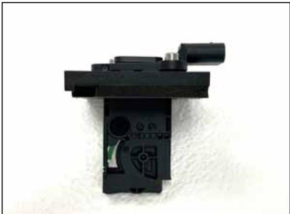
6. Install the provided gasket onto the K&N® MAF sensor adapter. Remove the MAF sensor from the factory housing and install it into the MAF sensor adapter and secure with the provided hardware.
