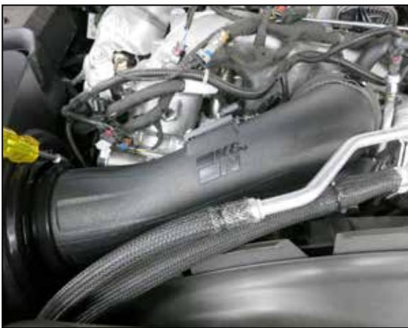
13. Install the K&N intake tube into the filter and then into the coupler at the turbo inlet, adjust the tube for best fit and then secure with the provided hose clamps.
