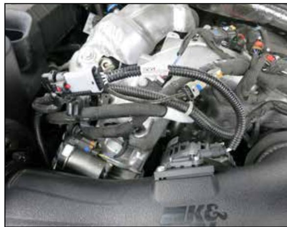
14. Connect the provided mass air sensor harness extension onto the mass air sensor and then connect the open end to the factory harness.
