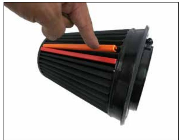
10. Attach the filter clips to the pleats on the air filter align and push down. Passenger side filters, place orange clip on top and red on bottom.
