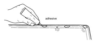
ATTACH AND ALIGN GASKET. Apply quick-drying adhesive sparingly in several places on the mating surface of cover. If gasket has installation tabs, adhesive is **not** reqiured. Mount gasket on cover. Allow time for adhesive to set. Test for slippage with light pressure if gasket moves, allow more time.
