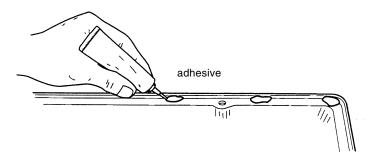
**ATTACH AND ALIGN GASKET.** Apply quick-drying adhesive sparingly in several places on the mating surface of cover. If gasket has installation tabs, adhesive is **not** reqiured. Mount gasket on cover. **Allow time for adhesive to set.** Test for slippage with light pressure if gasket moves, allow more time.
