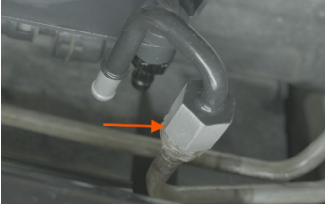
17. Install the MM1662 line assembly and connect it to the MM1513-15 fitting, MM1670 adapter, and the transmission cooler using the provided worm gear clamps. (4x MM1325-2) Then reinstall the grey plastic clip onto the transmission line fitting.
