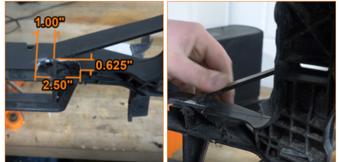
19. Trim the back of the grille support as shown in the below images.
