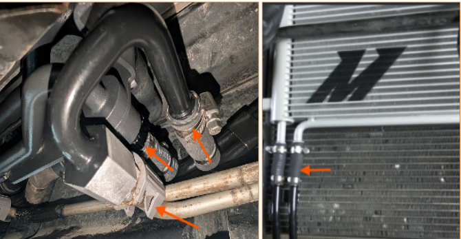
17. Install the MM1662 line assembly and connect it to the MM1513-15 fitting, MM1670 adapter, and the transmission cooler using the provided worm gear clamps. (4x MM1325-2) Then reinstall the grey plastic clip onto the transmission line fitting.
