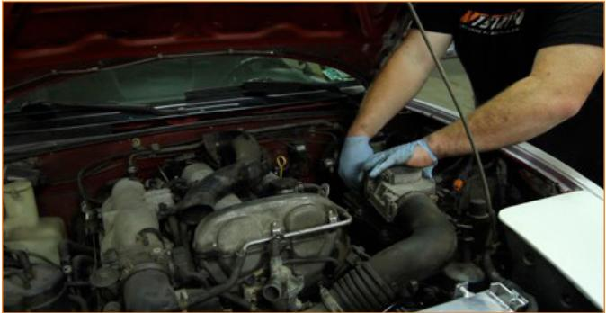
**3.** Reconnect the mass airflow sensor connection.
