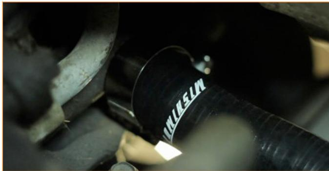
**2.** Reinstall the air box and OEM intake tubes by doing steps 2.1-2.3 in reverse. Make sure to securely tighten the 10mm bolts on the intake tubes, as well as the 12mm nuts on the air box.
