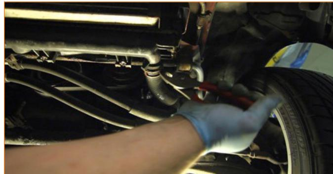
5. Working with care, carefully remove the factory heater hose on the right from the vehicle.
