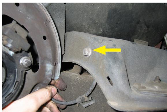
13. Move the ABS cable out from behind the upper control arm to prevent damage during the dust shield removal.
