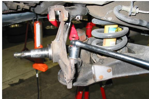
18. Loosen the upper ball joint 21mm nut with the same procedure as the lower, leaving the nut on the threads. Using the hammer method as above, loosen the upper ball joint from its position.
