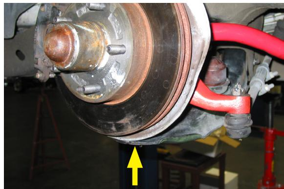
31. If there is severe "toe-out" in the wheel positioning, loosen the two 13mm nuts on the tie rod adjusting sleeves and turn them approximately 2 to 2.5 turns or until wheels appear straight. This will temporarily adjust the toe-in of the vehicle to enable you to drive the vehicle to an alignment shop. Tighten the tie rod clamp bolts and torque to 16 ft lbs.
