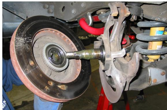
11. **For vehicles not equipped with ABS**, remove the dust cover from the spindle by removing the upper and lower 10mm bolts; and the 13mm bolt from the face of the cover. Detach the cover from the spindle and safely hang it behind the spindle.
