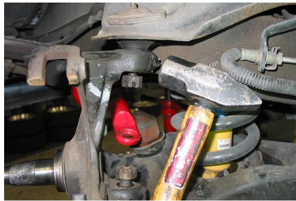
19. Once they are both loose, remove the upper nut and lift the control arm to free the spindle. Now remove the lower nut and slide the spindle off the lower ball joint.
