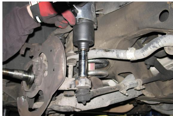
16. Place a floor jack under the lower control arm and lift until a slight compression of the suspension is achieved. Turn the spindle to access the lower ball joint without interference.
