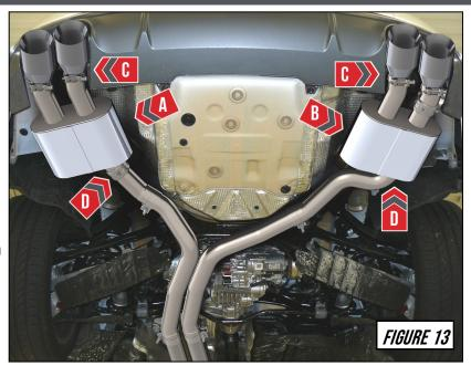
Plug the factory valve harnesses into the new valve control motors, shown by **Arrow D** in **Figure 13**. **NOTE:** If the AWE SwitchPath Remote Kit has been purchased, continue the installation process by downloading the next set of instructions **HERE**.
