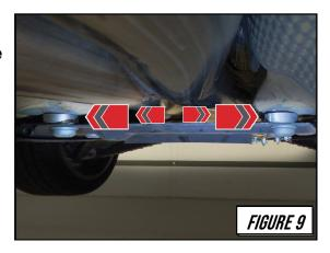
Failure to install the provided Brace Spacers properly may result in contact between the AWE mid-pipe and your driveshaft or cross brace.
