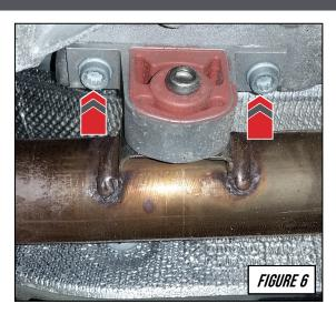
Install the downpipe upper sections (part A10 & A11) using the included flange gaskets and mounting hardware to secure them to the outlet flange of the factory catalyst.
