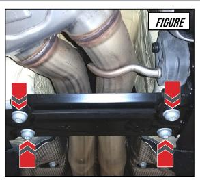
Starting from the rear of the car, support the OEM rear mufflers and loosen the four (4) 13mm bolts that secure the sleeve clamps into place, as shown by the arrows in **Figure 4**.
