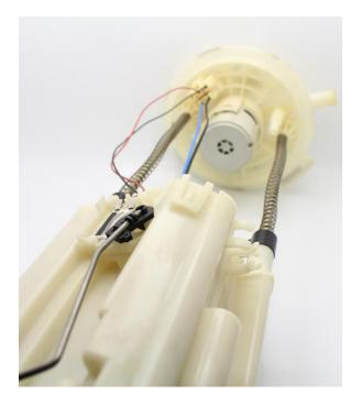
7 – reinstall the assembly into the fuel tank and attach a length of hose to the outlet of the pump assembly allowing it to drain into a fuel safe container and prime the fuel pump assembly
