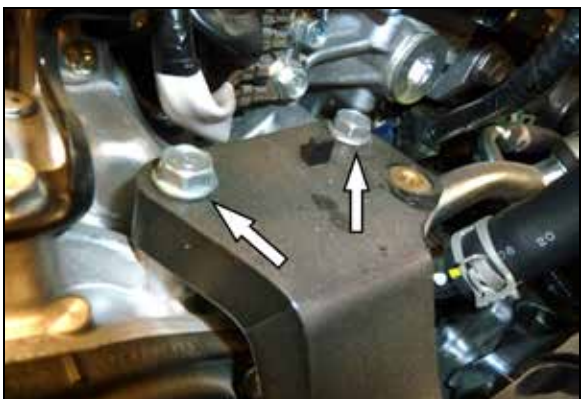
9. Remove the charge tube mounting bolts.
