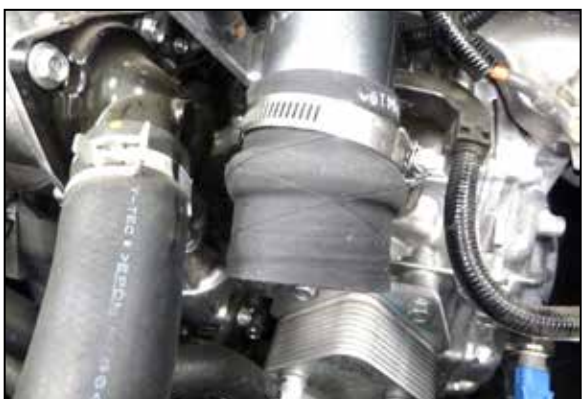
16. Install the provided step coupler onto the upper charge tube but do not secure.
