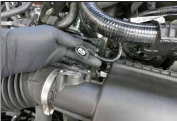
3. Disconnect the Mass Air Sensor electrical connection.
