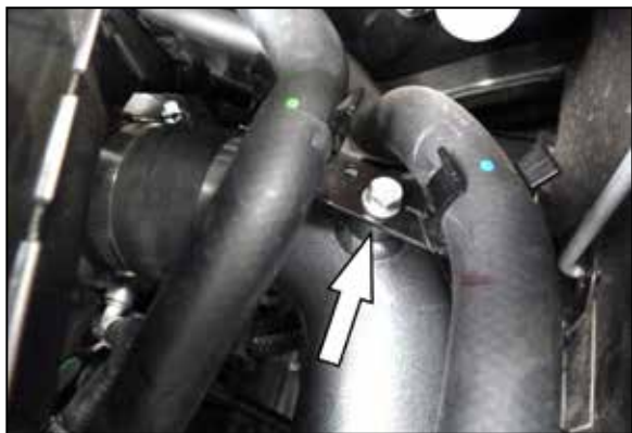
20. Install the factory hose holder onto the K&N charge tube and secure with the factory bolt.
