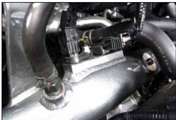
19. Connect the vacuum line to the npt fitting installed into the upper charge tube then reconnect the pressure sensor electrical connection.
