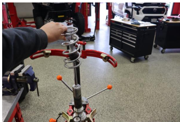
Step 10. Remove the OE tender spring.
