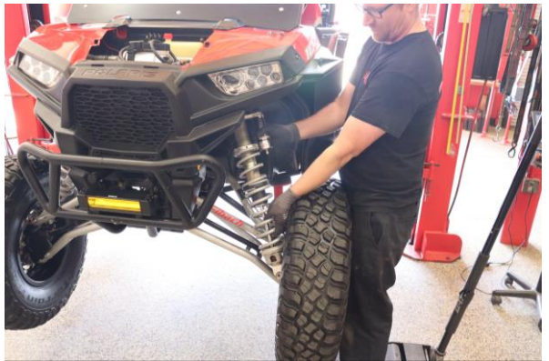
Step 16. Install shock assembly in the vehicle
