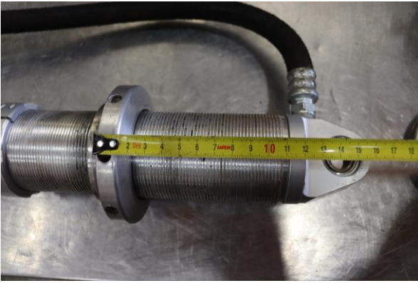
Step 13. Set pre-load to 115mm (4 1/2") from bottom of spring seat to bottom of reservoir bridge collar.
