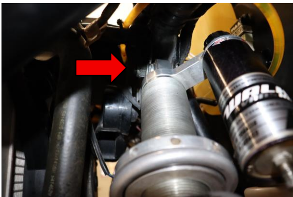
Step 17. Install upper shock mount nut and bolt loosely. Slightly lift on wheel and rotate lower shock
