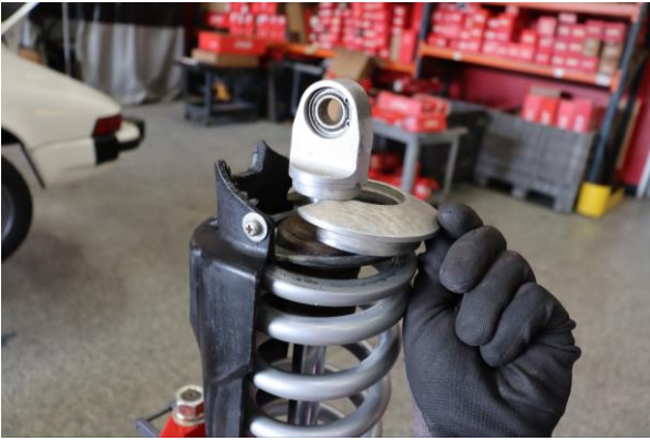
Step 19. Install the OE lower spring perch.
