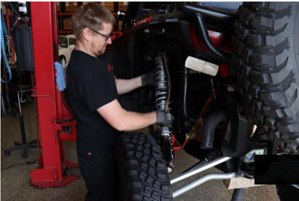
Step 21. Set the shock assembly in the vehicle.
