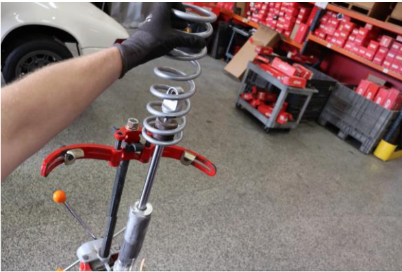
Step 15. Install Eibach tender spring.
