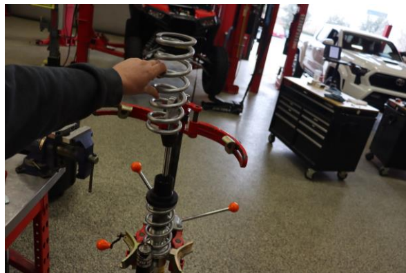
Step 8. Remove the OE main spring.
