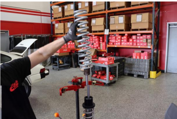
Step 17. Install Eibach main spring.
