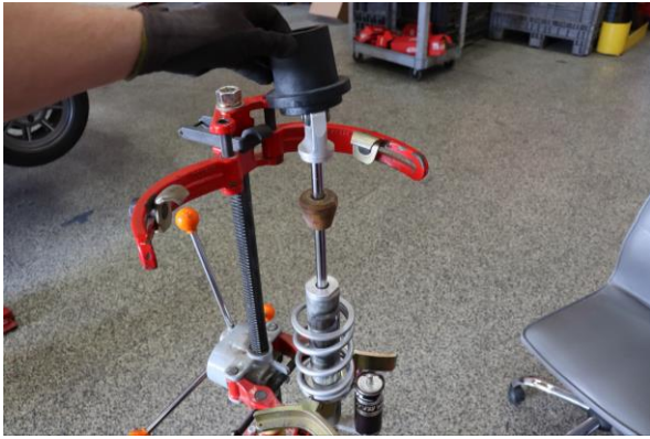
Step 13. Install Eibach front spring slider with the short end facing the top of the shock.
