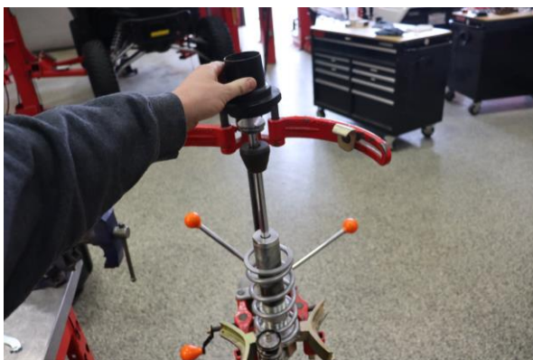
Step 9. Remove the OE spring slider.
