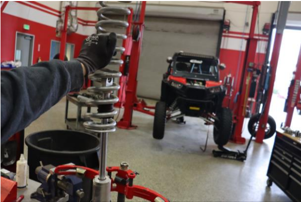
Step 9. Remove the OE main spring.
