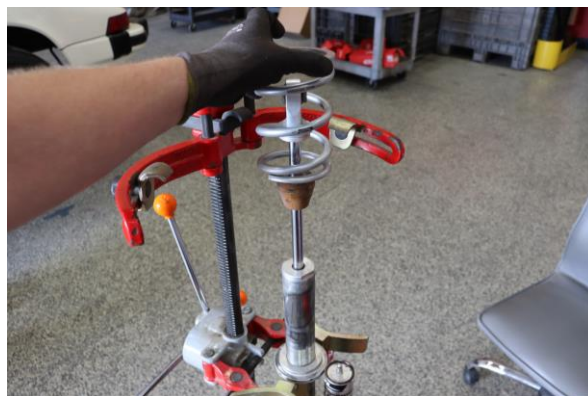
Step 12. Install Eibach front tender spring
