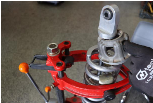
Step 15. Install OE lower spring perch. Decompress assembly and ensure lower spring perch engages lower shock mount fully.
