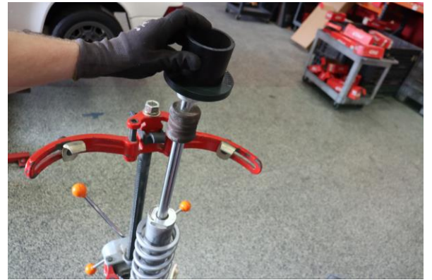
Step 16. Install Eibach spring slider with the short end facing the top of the shock.
