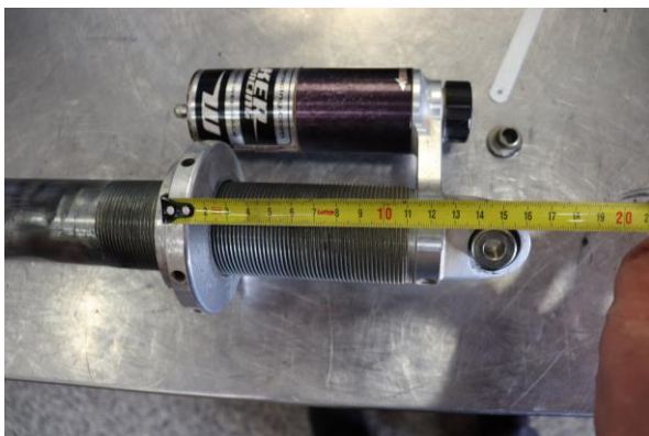
Step 11. Adjust the upper spring perch to 115mm (4 1/2") measuring from the spring seat to the bottom of the bridge collar to set spring preload.
