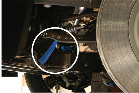
15. Begin from the driver side wheel and guide the sway bar into position above the front subframe. Again, do not damage the alternator pulley or AC lines.
