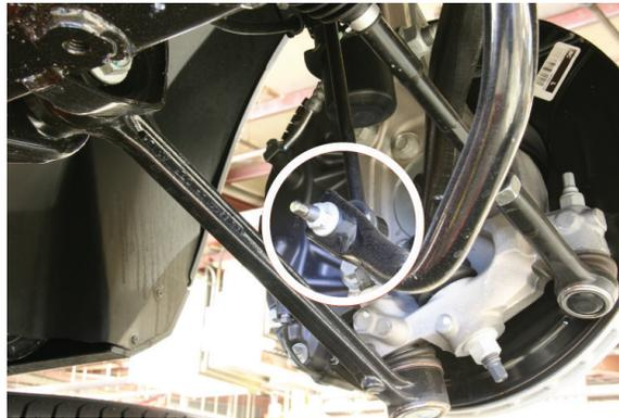
10. The pivot bushings and brackets are located on top of the front subframe, near the steering rack. Remove the four 13mm pivot bushing bracket nuts, then remove the bracket and bushings. Rest the sway bar on top of the subframe for now.
