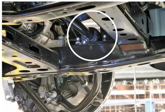
11. Break loose the two 18mm nuts that secure the engine mounts to the front subframe. Back the nuts off until only three to four full threads remain engaged.
