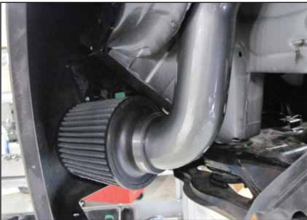
l. Install the AEM® Dryflow™ air filter.
