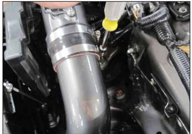
m. Ensure there is sufficient clearance around the intake tubes. Once proper fitment is achieved, tighten all hose clamps and hardware.
