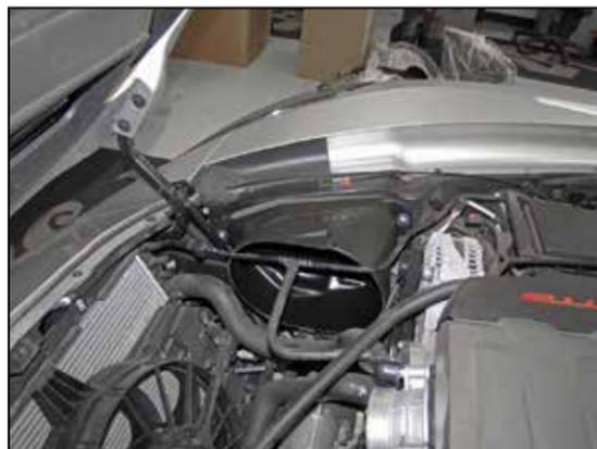
16. Install the AIRAID® air filter housing into the inner fender so that the mounting grommet engages with the mounting stud. Secure the housing with the provided hardware.
