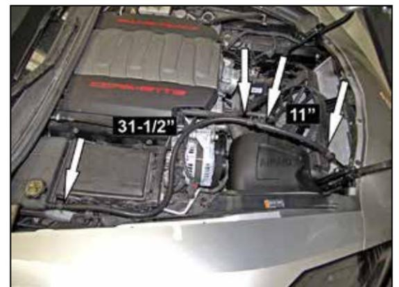
19. Trim the hose with the quick disconnect fitting to 31-1/2" long and trim the remaining hose to 11" long. Install the 31-1/2" long hose from the expansion tank to the tee fitting. Secure the hose with the provided spring clamp, route the hose as shown and secure with the provided tie wraps. Install the 11" hose onto the check valve and tee fitting and secure with the provided spring clamps.
