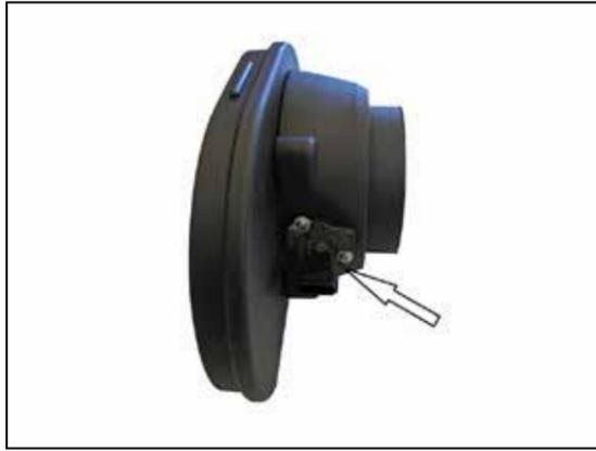
12. Remove the mass air sensor from the factory housing and then install it into the AIRAID® housing and secure with the provided hardware.
