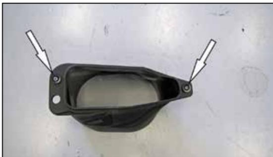
8. Insert the mounting grommets with sleeves into the AIRAID® air filter housing at the two locations shown.
