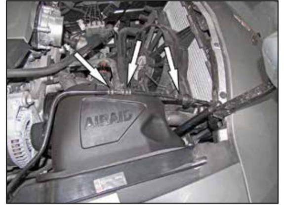
17. Be sure the vehicle is completely cool before beginning this step. Be sure to capture any coolant that leaks from the lines. Using a razor or sharp instrument, cut the nylon coolant lines in the three locations shown. Use multiple shallow cuts so as not to cut too deep and cause damage to the underlying fittings. Remove the nylon coolant lines from the check valve and tee fitting and expansion tank. The check valve should still be attached to the line attached to the radiator.
