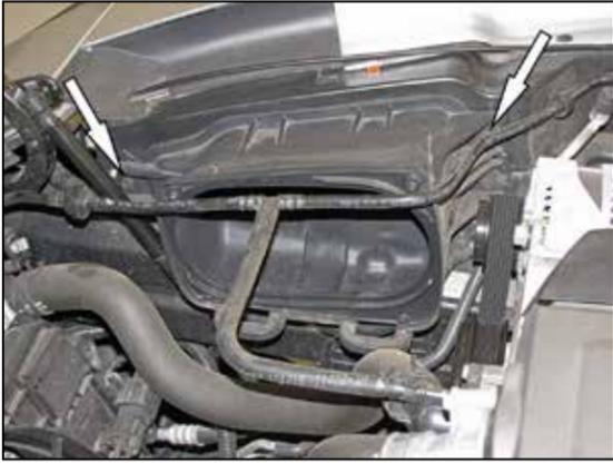
7. Remove the two bolts that secure the remaining air filter housing to the inner fender and then remove the housing from the vehicle.
