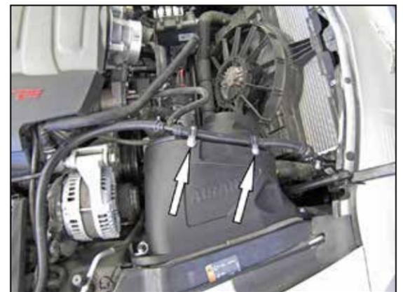
20. Install the AIRAID® filter assembly into the filter housing, install the provided loop clamps onto the coolant hose and then secure the filter assembly and coolant hose with the provided hardware.
