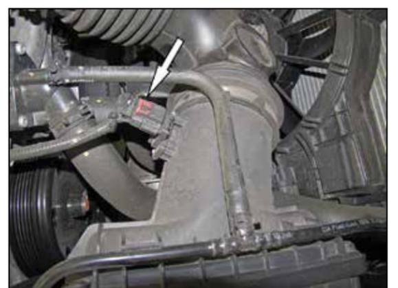
5. Slide the red tab back and then depress the mass air sensor locking tab and disconnect the mass air sensor electrical connection.
