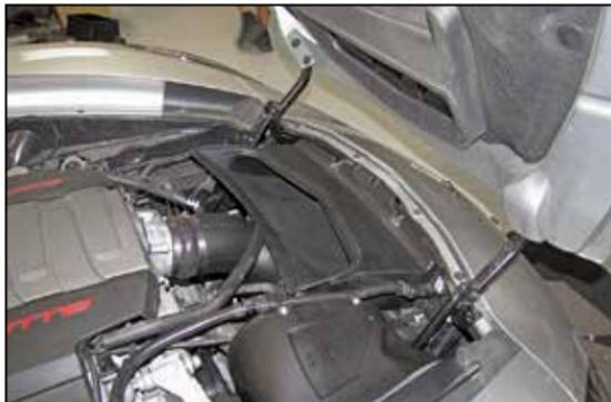
26. Reinstall the radiator heat extractor duct and secure with the factory hardware.
