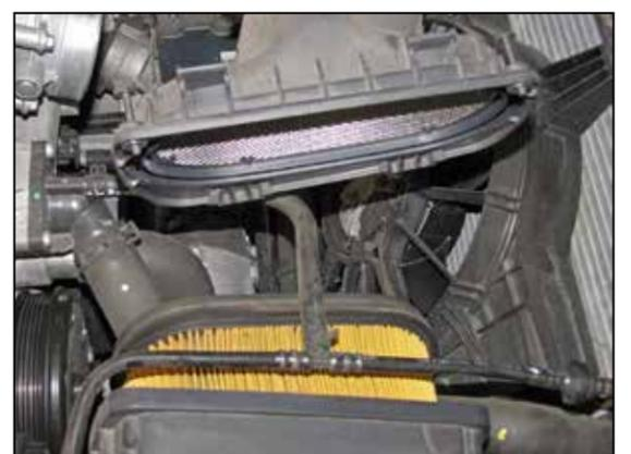
6. Unhook the coolant lines from the air filter housing, then loosen the two screws that secure the mass air portion of the air filter housing and remove it from the vehicle along with the factory air filter.
