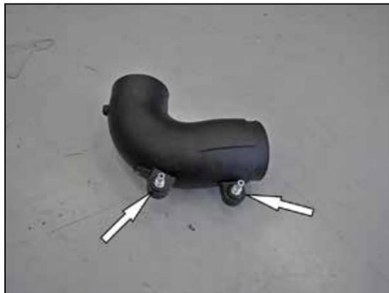
14. Install the provided grommets and crank case vent fittings into the AIRAID® intake tube as shown.
