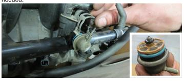
22. Using retaining clip pliers, install the fuel pressure regulator into the fuel pressure adapter.
