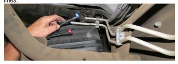
3. Disconnect the fuel tank EVAP line from the EVAP canister. Cap or tape up the fuel and EVAP lines to prevent possible system contamination.
