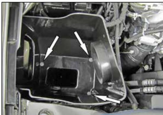
6. Install the AIRAID® Cold Air Box into the vehicle and secure to the air filter mounting plate location and secure with three of the factory bolts from step #4.
