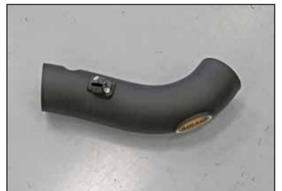
9. Install the mass air sensor into the AIRAID® intake tube and secure with the provided hardware. Install the AIRAID® decal to the tube.
