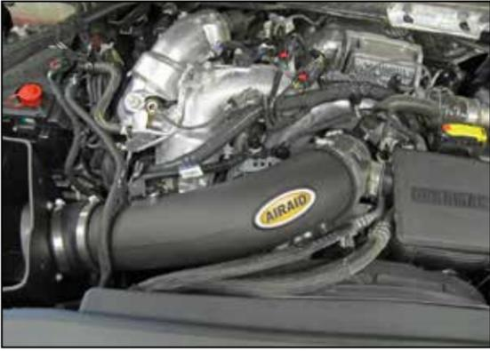
10. Install the AIRAID® intake tube into the elbow coupler and then into the factory plenum, adjust the elbow coupler and intake tube for best fit and then secure with the provided hose clamps.
