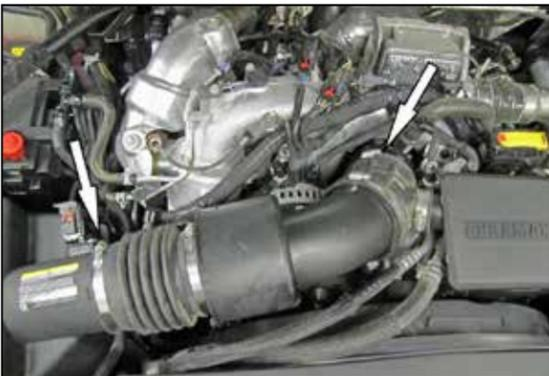
2. Loosen the hose clamps that secure intake tube to the turbo inlet and air filter housing, then remove the intake tube from the vehicle.
