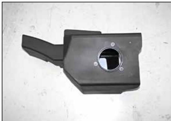
5. Install the provided air filter adapter into the AIRAID® Cold Air Box and secure with the hardware provided.
