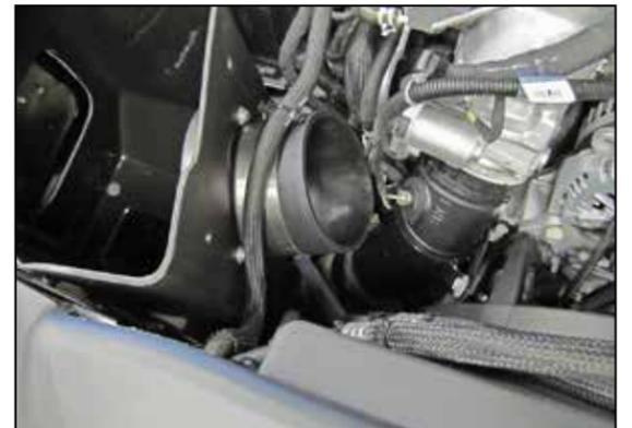
7. Install the elbow coupler hose clamps onto the filter adapter as shown but do not tighten at this time.
