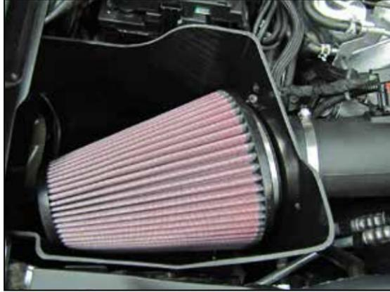
12. Using care so as not to damage the air filter, Install the AIRAID® air filter into the air box and onto the filter adapter, then secure with the provided hardware.
