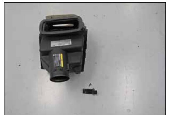
8. Remove the mass air sensor from the factory air filter housing as shown.
