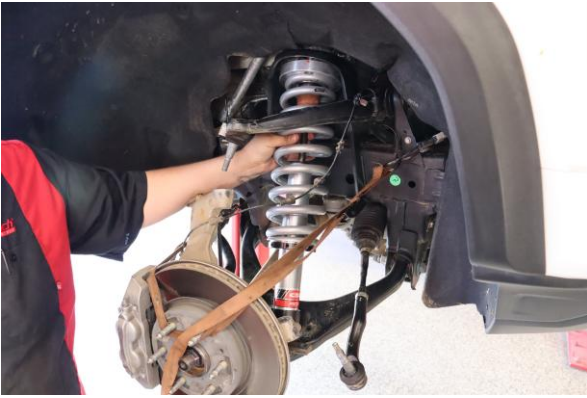
Step 13. Install the Eibach coilover assembly in the vehicle.
