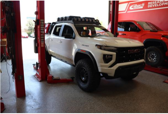
Step 1. Lift and support vehicle.
