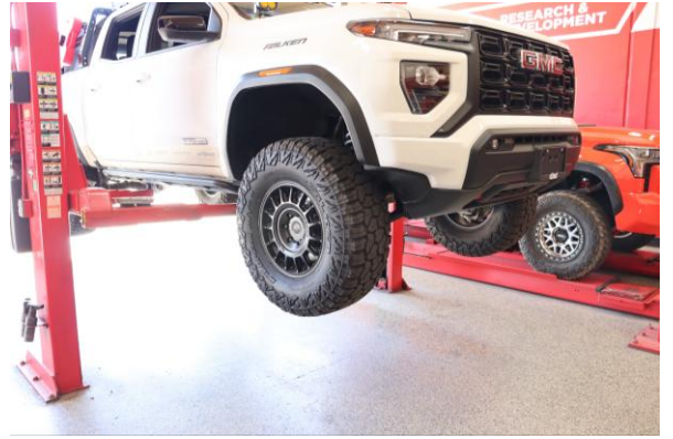
Step 2. Remove front tire using 21mm.
