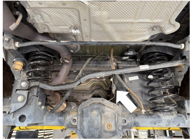
Fig. 35a: Route right rear shock harness, plug RRC connector into rear right shock
