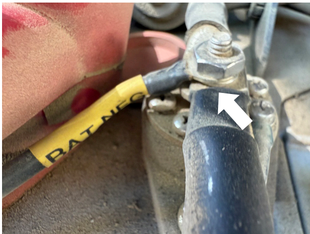
Fig. 39b: Connect GND BATT to ground terminal
