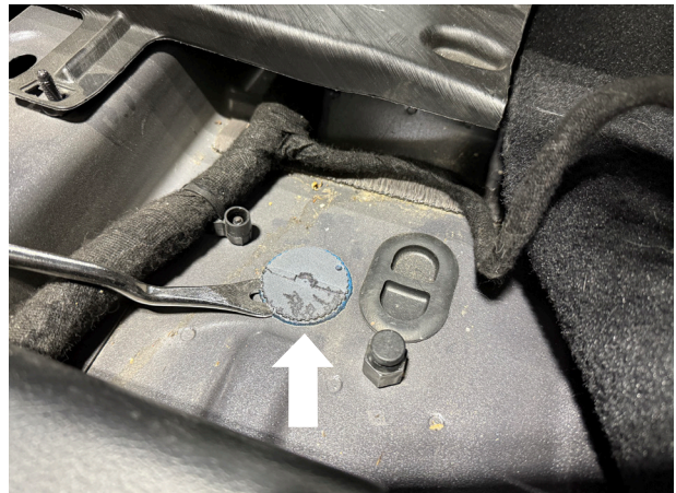
Fig. 14: Remove/pry grommet out.
