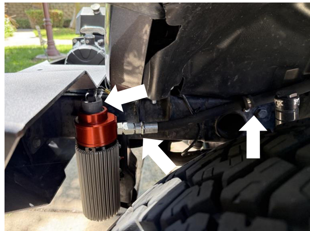
Fig. 37: Plug the FLC connector into the front left shock
