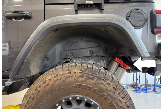
Fig. 36a: Route left rear shock harness, plug RLC connector into rear left shock
