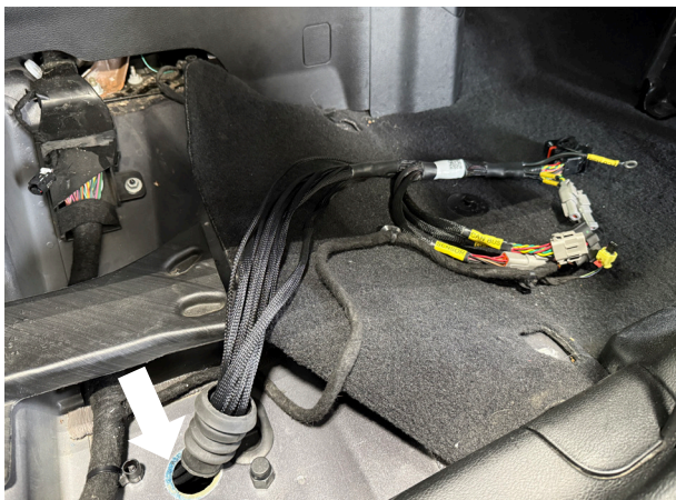
Fig. 19: Pass wires through cab floor.
