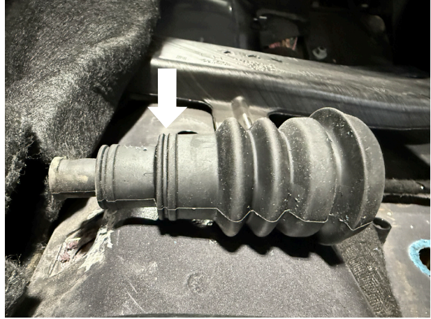
Fig. 16: The 026-01-298 grommet before modification.
