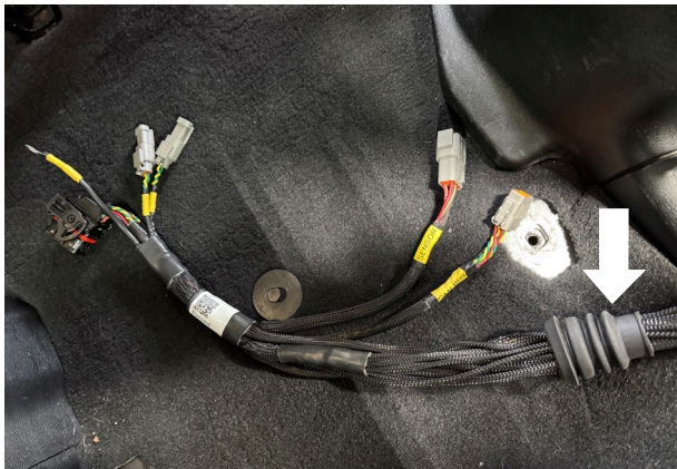
Fig. 18: Assemble grommet onto harness.
