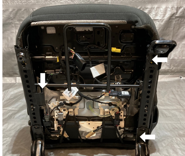
Fig. 9a: Identify the three tabs for mounting the bracket.
