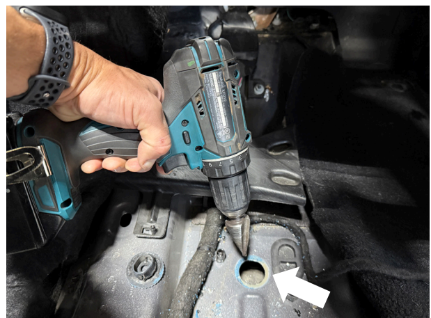
Fig. 15: Open up grommet hole to 1.125".
