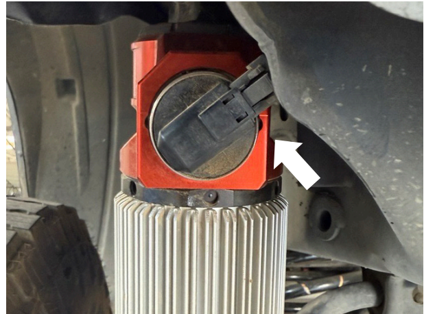
Fig. 36c: Route left rear shock harness, plug RLC connector into rear left shock
