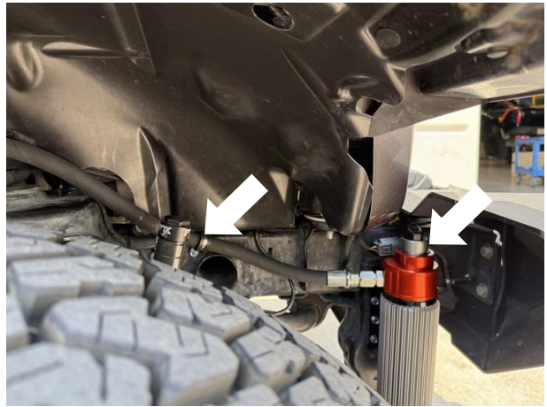
Fig. 41: Plug FRC connector into front right shock
