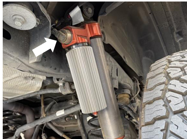
Fig. 35c: Route right rear shock harness, plug RRC connector into rear right shock
