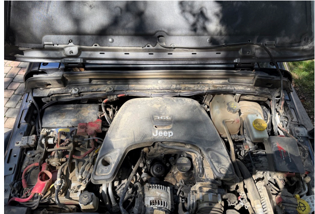
Fig. 38: Route power harness and front right shock harness
