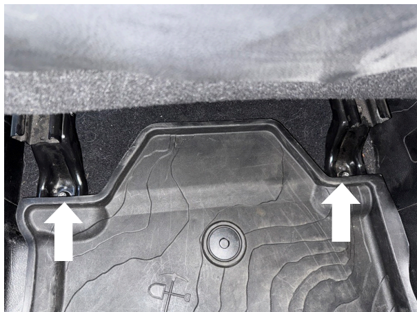
Fig. 1: Remove the two rear bolts.
