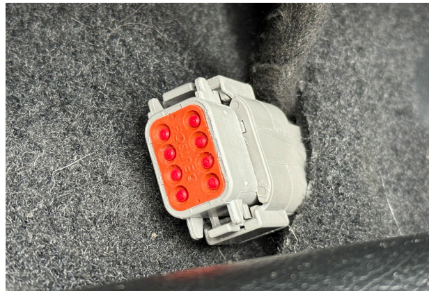
Fig. 25: 8-pin dust cap (218-02-102) on the “ROTARY” branch 8-pin connector
