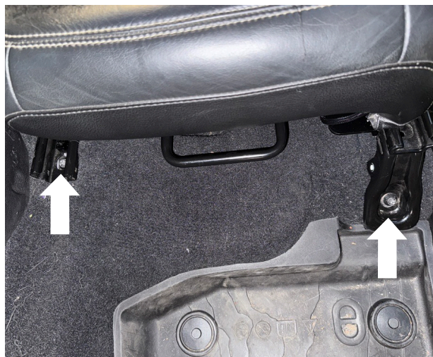
Fig. 2: Remove the two front bolts.
