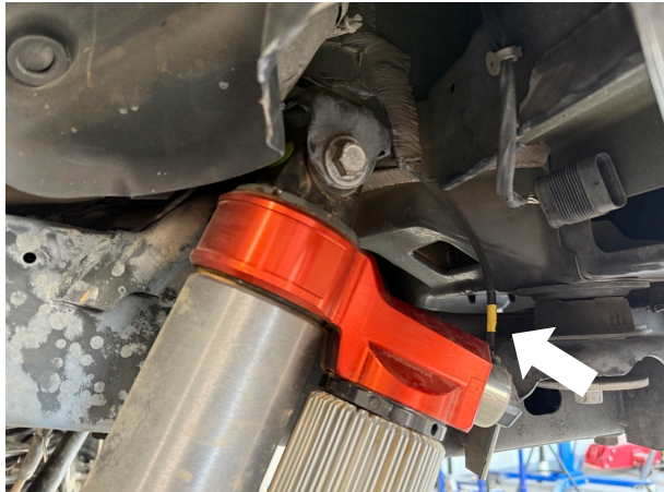
Fig. 36b: Route left rear shock harness, plug RLC connector into rear left shock
