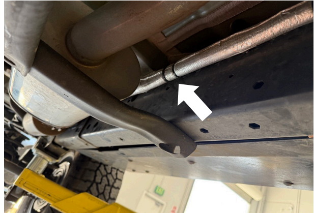
Fig. 34a: Secure rear shock harnesses
