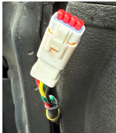
Fig. 26: 4-pin dust cap (218-02-103) on the “TOUCHPOINT” white 4-pin connector
