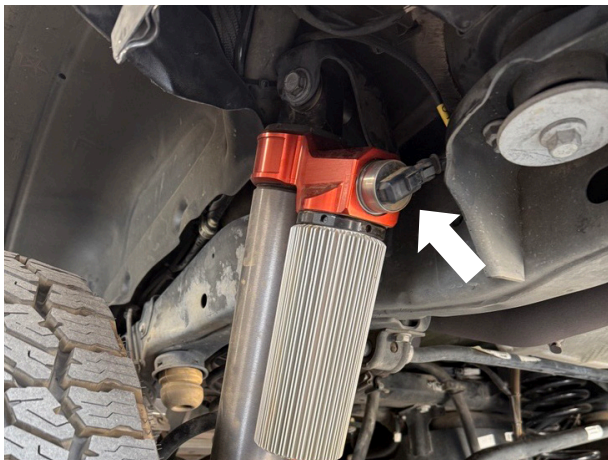
Fig. 36d: Route left rear shock harness, plug RLC connector into rear left shock
