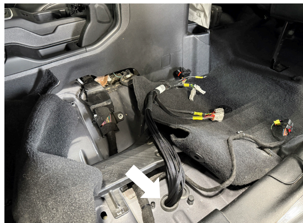
Fig. 20: Install grommet in cab floor
