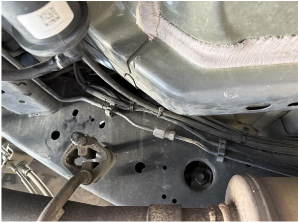
Fig. 34b: Secure rear shock harnesses
