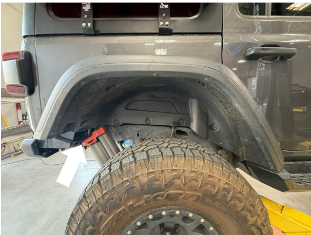
Fig. 35b: Route right rear shock harness, plug RRC connector into rear right shock
