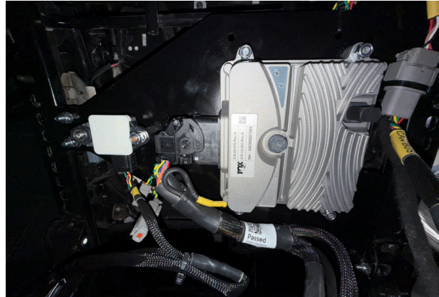
Fig. 32: Connect the 48-Pin connector on main harness (218-02-083) to the ECU
