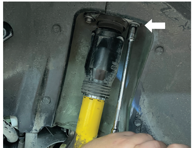
Fig. 16: Remove the upper shock bolts.
