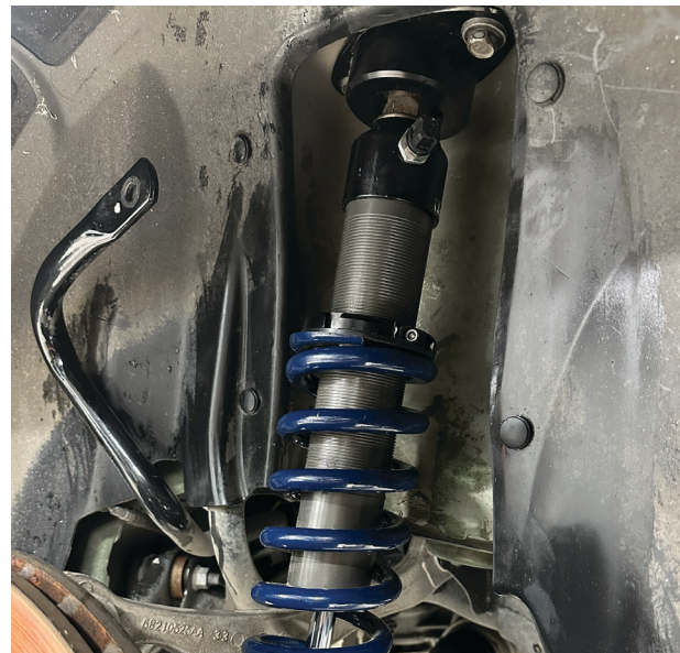
Fig. 21b: Install the new shock assembly; adjuster facing inboard, larger spacer to front of vehicle.
