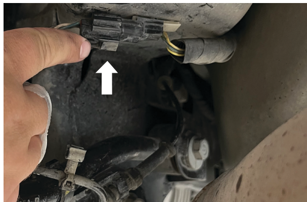
Fig. 12: Remove the clips for vehicles with adaptive damping system.
