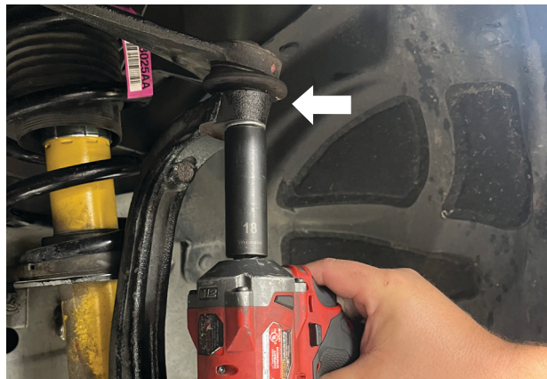
Fig. 7: Remove the upper ball joint.
