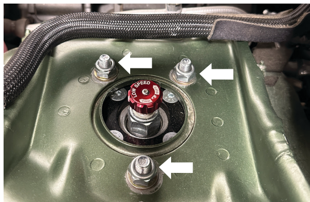
Fig. 10: Torque the top hat nuts on from engine bay.
