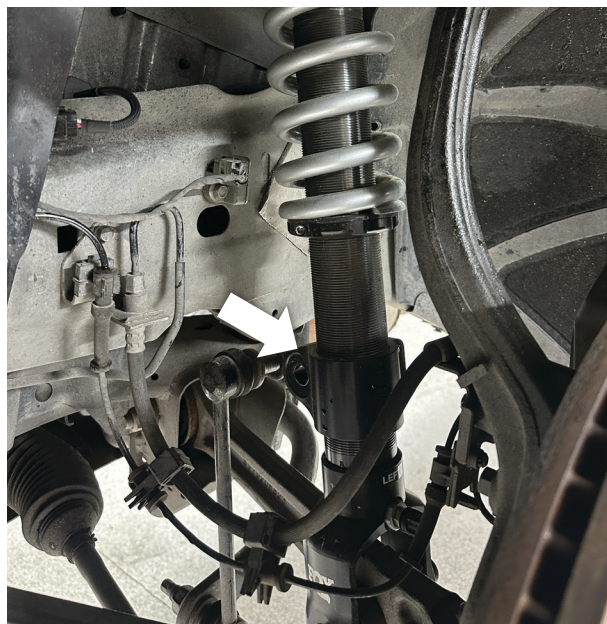
Fig. 9: Install shock with the sway bar mount facing inboard.
