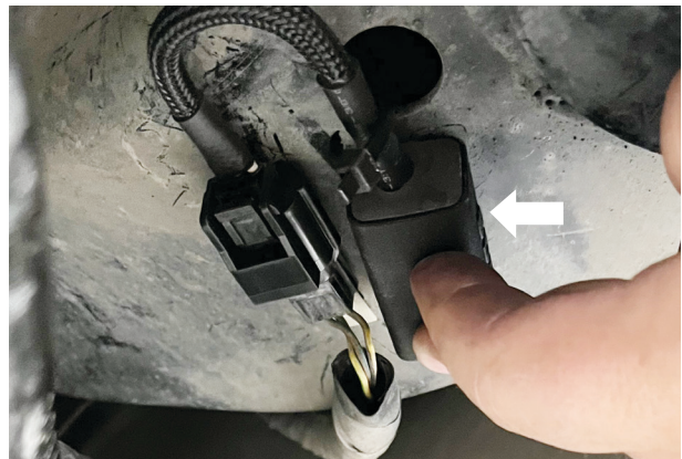
Fig. 23: If applicable, connect the adaptive damping system connector.
