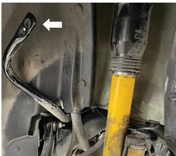
Fig. 14: Swing the sway bar out of the way, remove the stock bolt.
