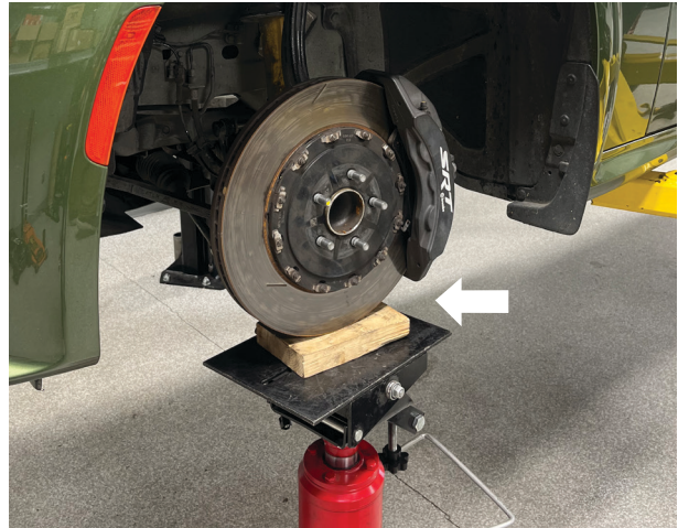
Fig. 6: Support the suspension.
