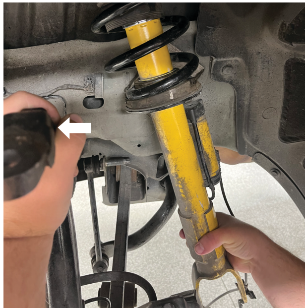
Fig. 8: Hold the spindle, remove the shock.
