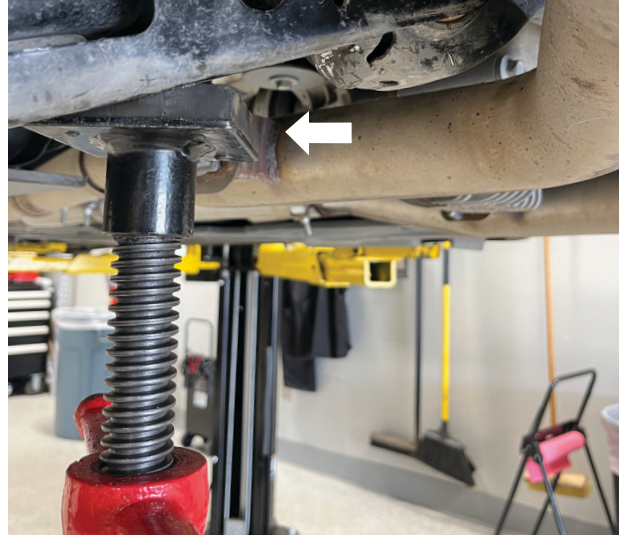
Fig. 18: Move the suspension support to the inside of the lower control arm.
