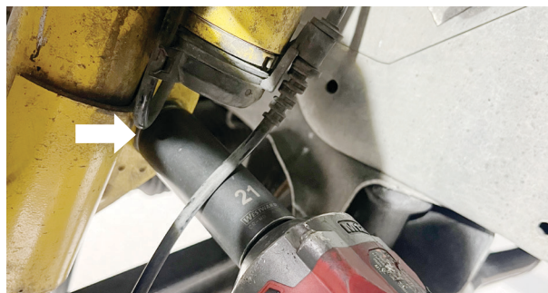
Fig. 2: Remove the sway bar nuts.
