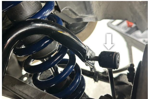
Fig. 22b: Reinstall stock sway bar hardware; bolt outboard.
