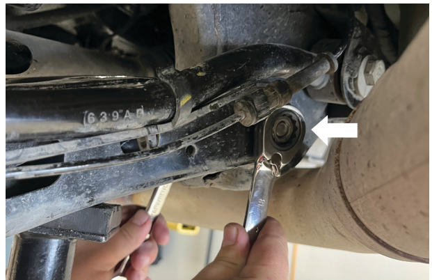
Fig. 19: Remove the inner lower control arm bolt.
