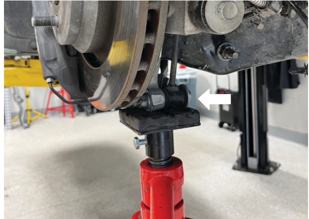
Fig. 15: Support the suspension toward the outside of lower control arm.
