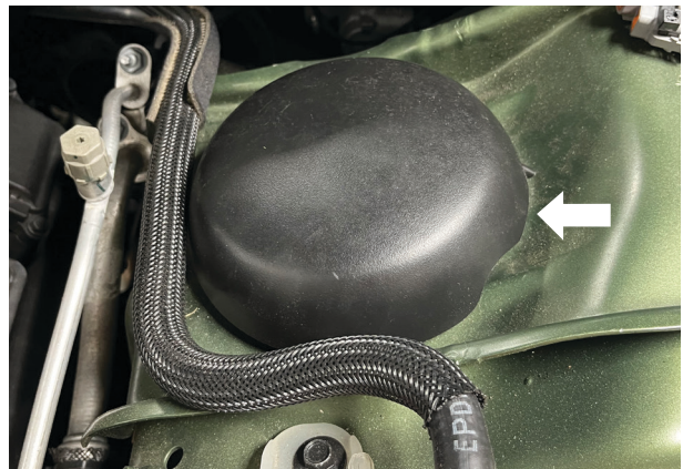
Fig. 4: Remove the black cap.
