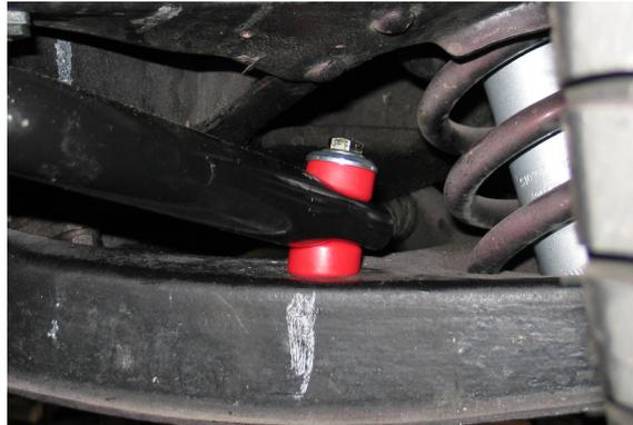
14. With the end links attached to the control arms, place the supplied pivot bushings and pivot bushing brackets onto the sway bar without lubrication. Position them directly under the frame. Use the brackets to mark the position of the four mounting holes. Center punch the marked locations and drill four 3/8" diameter holes.
