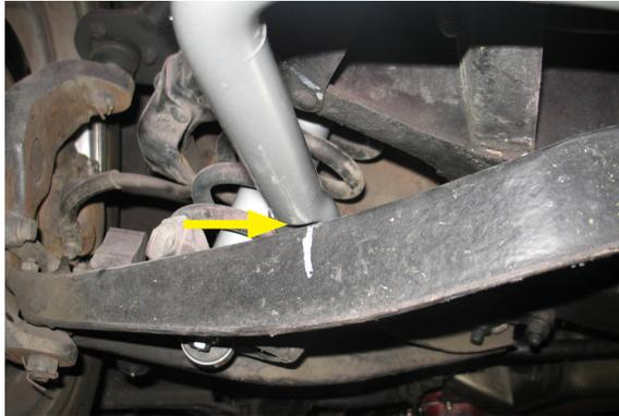
10. After the holes have been marked, measure the distance between the end link hole centers of the sway bar and compare the distance between the two marked points on the control arms. They must be the same.
