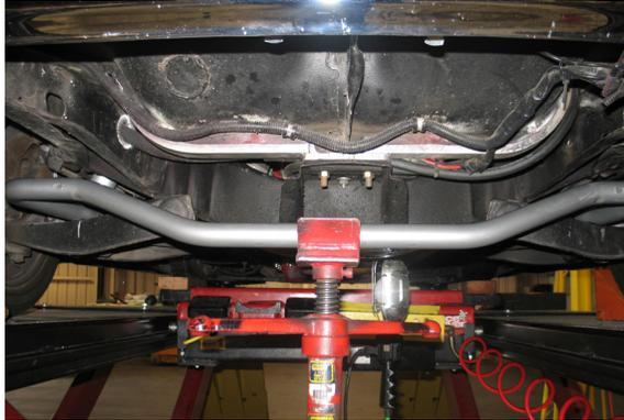
9. Use the ends of the sway bar to mark the lower control arms where new holes will be drilled for the end links.
