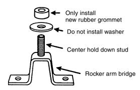
**INSTALL A NEW RUBBER GROMMET SEAL** on each center hold-down stud (see drawing).
