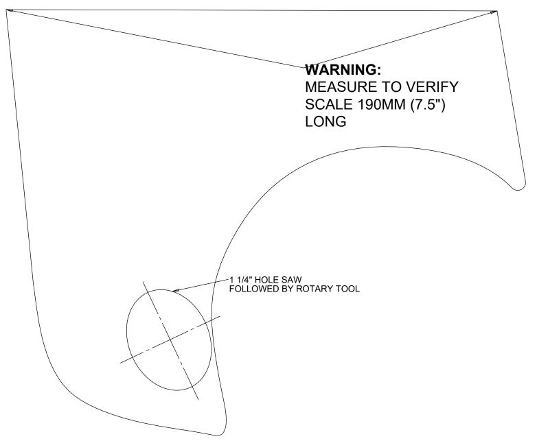
PLACE DRILLING TEMPLATE ON INSIDE OF FOG LIGHT COVER, ABOVE AND NEXT TO LIGHT CUTOUT
