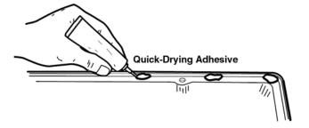
**ATTACH AND ALIGN GASKET.** Apply quick-drying adhesive, sparingly in several places on the mating surface of cover. If gasket has installation tabs, adhesive is **not** required. Mount gasket on cover. **Allow time for adhesive to set.** Test for slippage with light pressure. If gasket moves, allow more time.
