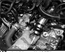
**17.** Install the provided 2.25" hump hose with clamps provided to the upper intercooler pipe. Do not tighten.
