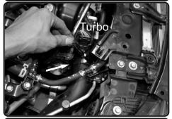
**22.** Loosen the clamp on the turbo using 10mm socket or wrench. Pull back the hose from turbo.
