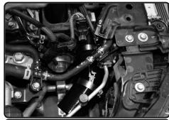
**27.** Install the provided elbow hose to the turbo using clamps provided. Do not tighten. Install the injen intercooler pipe into vehicle.
