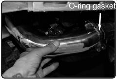
**28.** Install the injen intercooler pipe into vehicle.
