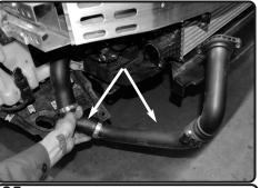
**25.** Carefuly remove the hot side intercooler pipe out of vehicle.
