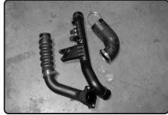
**11.** Complete cold side of intercooler pipe removed.
