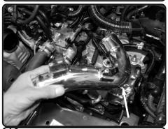
**16.** Install upper intercooler pipe into the vehicle and position to the hump hose. Do not tighten.
