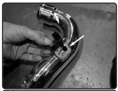
**14.** Install the upper temperature sensor with provided M5 screw and tighten.
