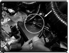
**5.** For easier removal, disconnect temperature harness on engine and pull back the entire harness from the cold side intercooler pipe.
