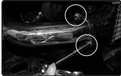
**29.** REMOVE FACTORY O-Ring gasket from OEM intercooler pipe and install to the new injen intercooler pipe. Connect the intercooler pipe flange to the intercooler using OEM bolts from step 24.
