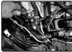
**23.** On back side of hot side intercooler pipe, locate the bolt holding in the intercooler pipe to bracket. Loosen and remove using 10mm socket and ratchet.
