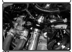
**20.** Adjust for the best fit, and tighten all clamps using 8mm nut driver.
