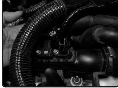
**3.** Disconnect both sensors on the upper intercooler tube.
