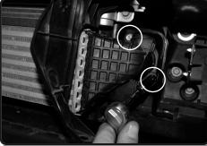
**9.** With front Bumper cover removed, Loosen and remove the 2 bolts holding in the lower intercooler pipe. Save for later install.
