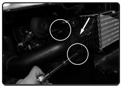
**24.** With front Bumper cover removed, Loosen and remove the 2 bolts holding in the lower intercooler pipe. Save for later install.
