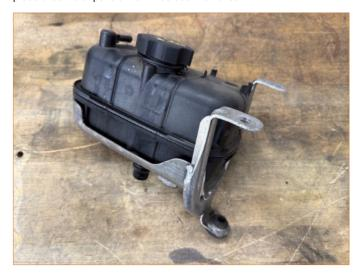
**5.** Remove the mounting grommet from the stock expansion tank and install it onto the Mishimoto expansion tank in the same orientation.
