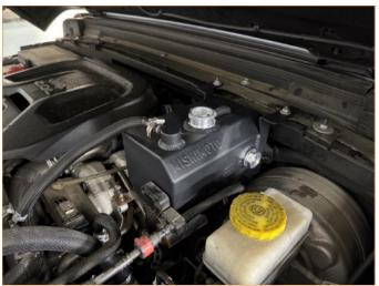
6. Connect the lower hose to the Mishimoto expansion tank and install the tank into the vehicle. Re-install the two mounting nuts, reconnect the upper hose using the included worm gear clamp, and reconnect the plastic brake vacuum line mount.
