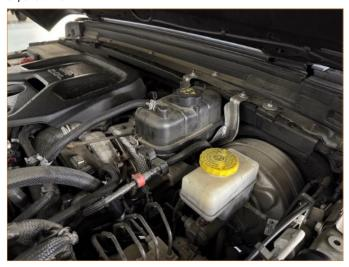
3. Using a pry tool, remove the plastic mount that attaches the brake vacuum line to the expansion tank. Disconnect the upper hose and the two nuts securing the expansion tank to the body of the vehicle.
