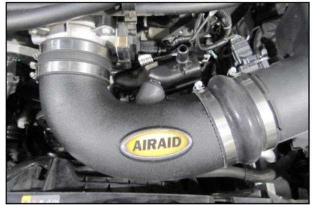
12. Insert the Intake Tube into the coupler first, then into the Hump Hose. Tighten all four clamps at this time.
