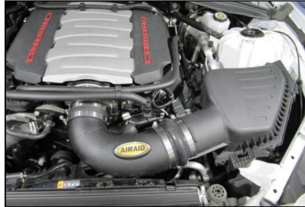
14. Slowly lower the hood to test clearances. Make sure all clamps, hoses, bolts, and screws are tight. Double check the hood clearance. Reconnect the negative battery terminal and re install the access panel.
