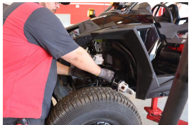
Step 6. Rotate shock out of upper and lower mounts and remove from the vehicle.
