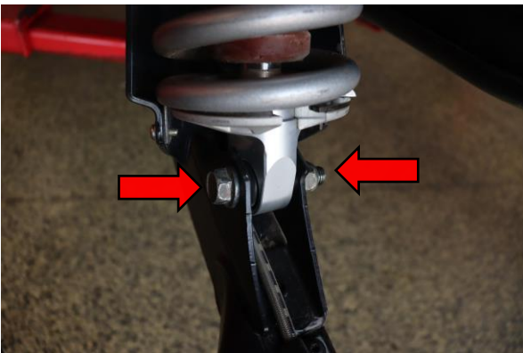
Step 23. Install the lower shock mount nut and bolt. Use two 18mm to tighten to manufacturer specification.
