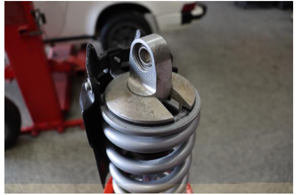
Step 20. Decompress the shock assembly ensuring the lower spring perch fully engages the lower shock mount.
