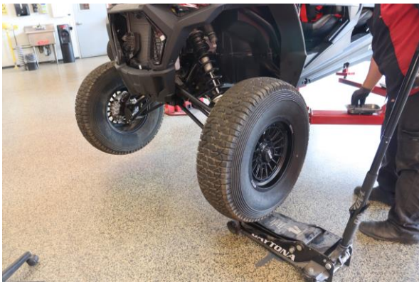
Step 3. Use a jack if vehicle is lifted on rack. Use a strap between the lower control arm and the frame to prevent damage to the axle from over extension.
