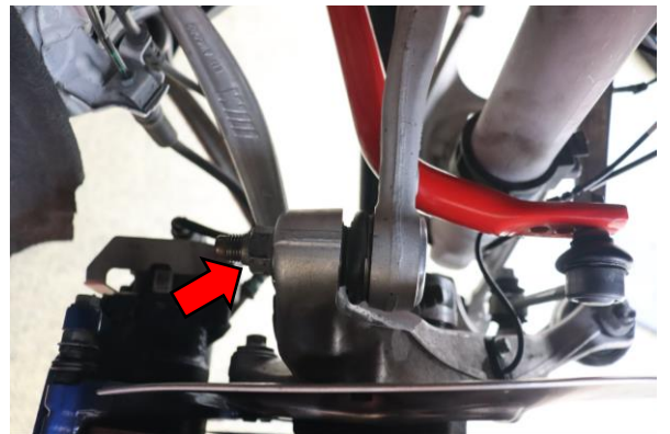
Step 24. Install outer mounting nut and tighten to manufacturer spec using a 21mm. Tighten inner control arm to mounting nut and bolt to manufacturer specification using two 16mm.
