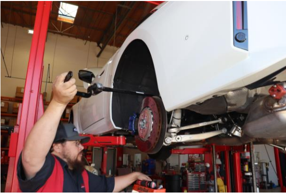
Step 19. Remove the rear sway bar from the left side of the vehicle. Be careful to not damage any wiring during removal.
