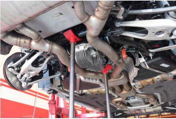
Step 25. Lift subframe into position. Periodically check to ensure no wires are being pinched.
