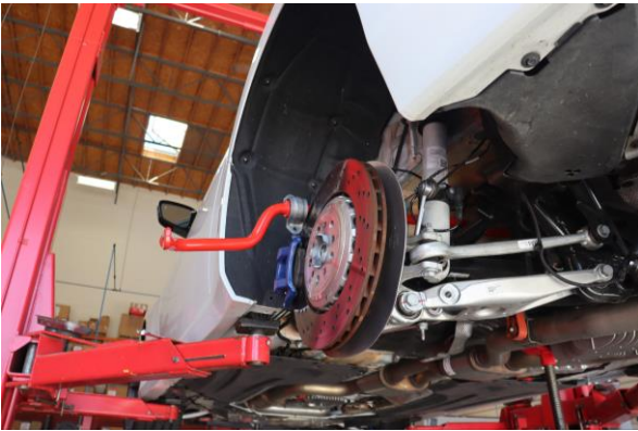
Step 21. Install new sway bar through the left side of the vehicle. Be careful not to damage any wiring during install.
