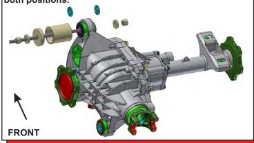
Passenger side frame bushing, front position. Do not remove outer metal shell. Old rubber bushing is not bonded to outer metal shell. Install 01P01345 with 15.10.135.39 into this
