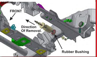
Passenger side frame bushing, rear position. Do not remove outer metal shell. Old rubber bushing is not bonded to outer metal shell. Install 01P01346 with 15.10.534.39 into this position.
