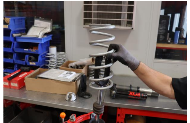
Install Eibach main spring
