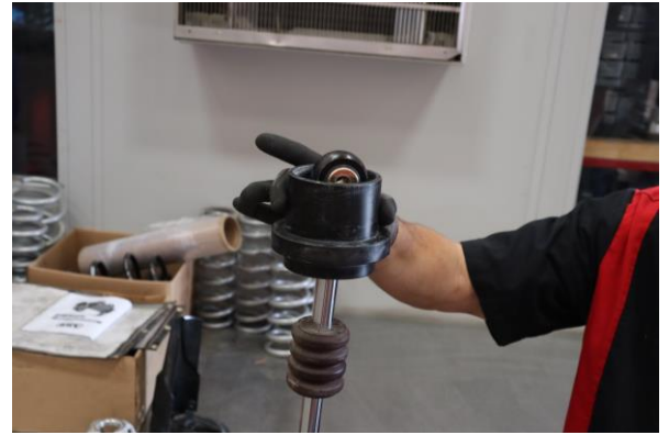
Install OE slider and Eibach main Spring
