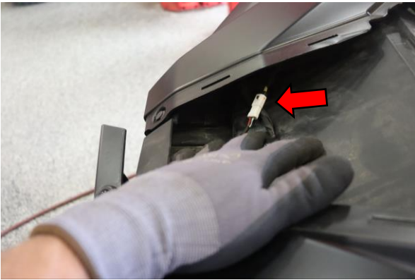
The front camera is attached to this assembly. Unplug and set aside.
