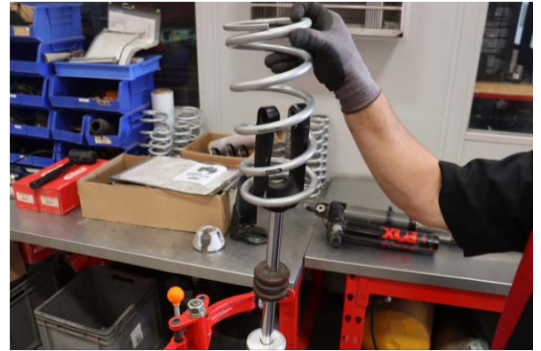
Install the Eibach secondary spring.
