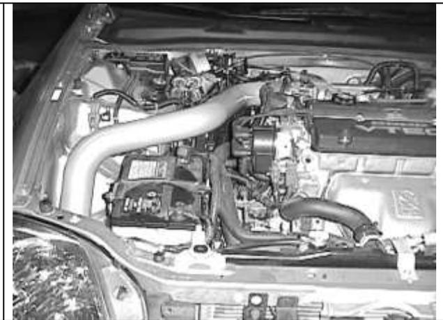
Fig 8: Intake tube installed
