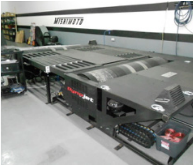
FIGURE 2: A Dynojet™ dynamometer was used for vehicle testing.
