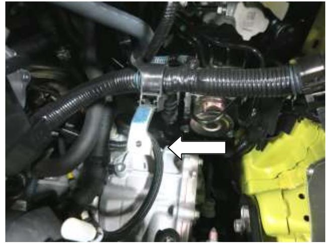
h. Remove the M6 bolt that secures the wiring harness to the lower air box and remove the lower air box.
