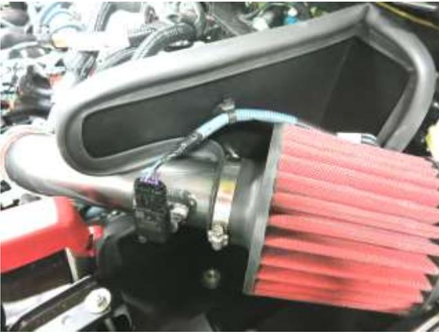
k. Reconnect the MAF sensor and secure the wiring harness clip to the heat shield as shown.
