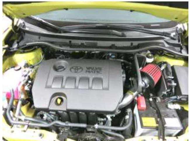
n. AEM 21-776C intake system installed.
