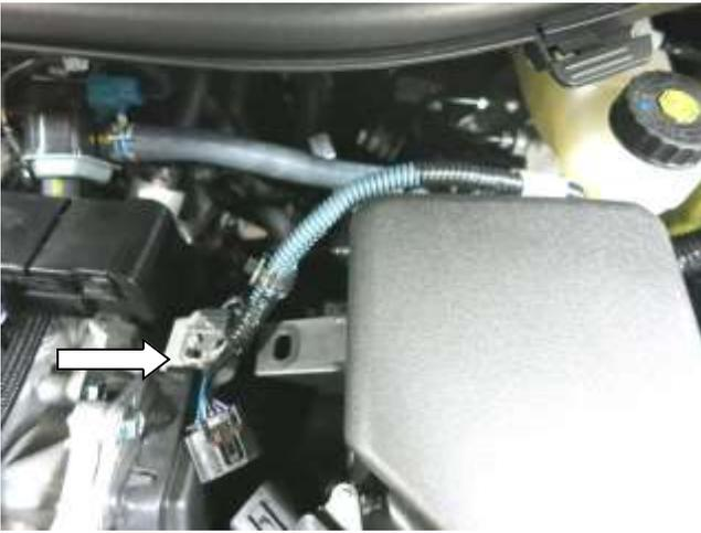
e. Release the clip that secure the MAF sensor wiring harness to the air box.
