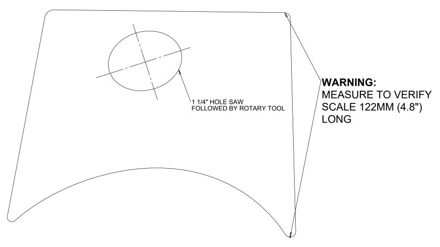
PLACE DRILLING TEMPLATE ON INSIDE OF FOG LIGHT COVER, ABOVE LIGHT CUTOUT
