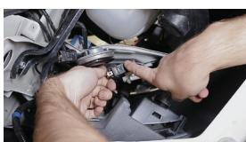
2. Once removed, pull down on the panel to gain access to the DRL resistor. The connector you need will be black and brown in color.
