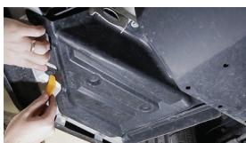
1. To begin, remove the three locking screws on the bottom wheel well panel located under the bumper on the passenger side of the vehicle.
