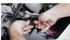
3. Unclip the connector from the body piece it is attached to by pushing straight out to release it.
