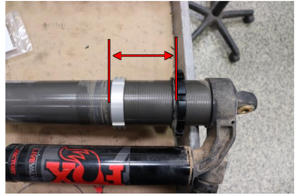
Step 14. Adjust the Eibach supplied crossover ring to 100mm (3 15/16") from bottom of spring seat to bottom of crossover ring.
