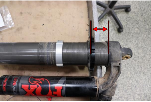
Step 13. Set pre-load to 60mm (2 3/8") from bottom of spring seat to bottom of reservoir bridge collar.
