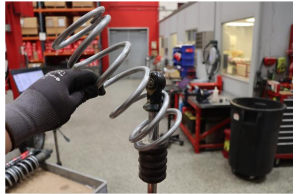
Step 16. Install the Eibach secondary spring.
