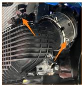
17. Release the intercooler from the radiator by pulling down on the lock tabs and then pulling forward on the bottom of the intercooler. Remove the intercooler by lifting the whole assembly up over the hooks on the radiator then removing it out the front. Note: you may have to lift the AC condenser a bit to gain more room.
