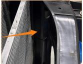
14. Remove the 4 bolts for the 2 radiator brackets then, remove the brackets.
