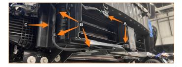
10. Remove the 4 bolts fastening the grill shutter assembly and the 4 bolts for the lower brace (8mm socket).
