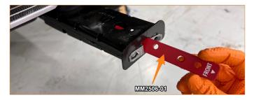
21. Through the 2 holes on the bottom of the frame, use your fingers to align the tie-down plate as shown. Hold it against the inside of the frame tube and install one of the supplied tree clips through the frame into the plate to secure it. Repeat for the other side of the vehicle.
