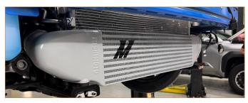
23. Line up the holes in the tie-down plate with the threads in the rubber mounts, then fasten the intercooler using the provided M6 hardware (4mm hex key). Repeat for the other side of the vehicle.
