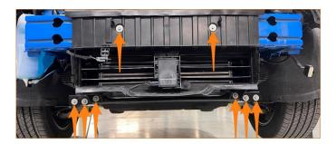
11. Unplug the electrical connector "A", remove the 3 harness tree clips "B", and remove the 2 bolts "C" (8mm socket). Remove the grill shutter assembly and the lower brace from the vehicle.
