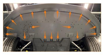
2. Remove the 6 pop clips from the left side wheel liner. Repeat this for the right side, then remove the splash guard from the vehicle.
