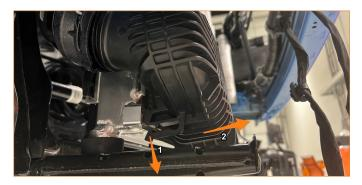
18. Remove the screw (T30 Torx) fastening the pressure sensor to the stock intercooler and remove the sensor. Install the sensor into the Mishimoto intercooler and fasten it using the provided M6 locking bolt (4mm hex key).
