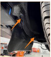
**3.** On the inside of the front bumper, unplug the marker lights (one on each side) and the front bumper harness connector.
