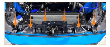
7. Behind the grill shutters and in front of the radiator, remove the screw for the grill shutter link (5.5mm socket), then bend the 2 tabs out on the bottom end and remove the link.
