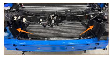
13. Remove the 2 tree clips (left) then remove the 2 plastic ducts (left and right).
