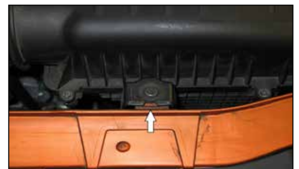
5. Remove the bolt holding in front of the airbox and save for later install.
