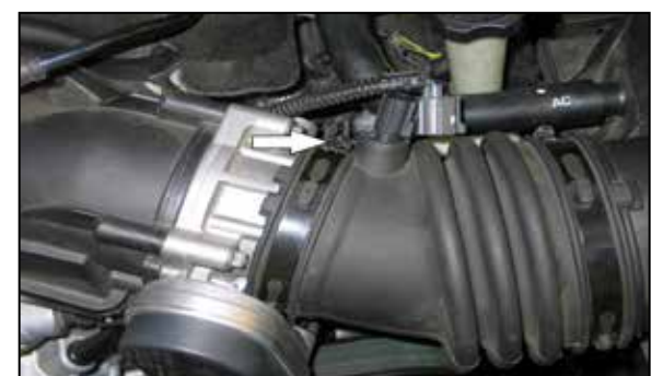
4. Loosen the clamp on the throttle body. Disconnect the Temperature sensor harness.
