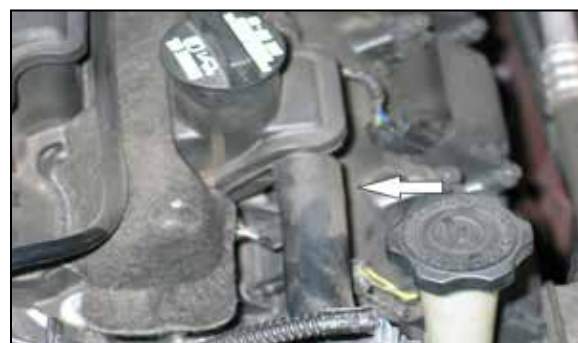
3. Locate the rubber Crankcase line and pull away from the engine.
