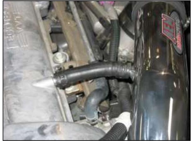
h. Secure the stock breather hose to the intake pipe nipple using the stock hose clamp.
