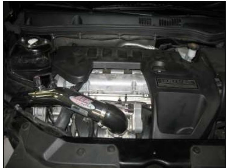
AEM® intake system installed
