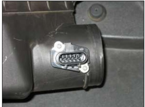
f. Remove the MAF sensor from the factory air box lid.
