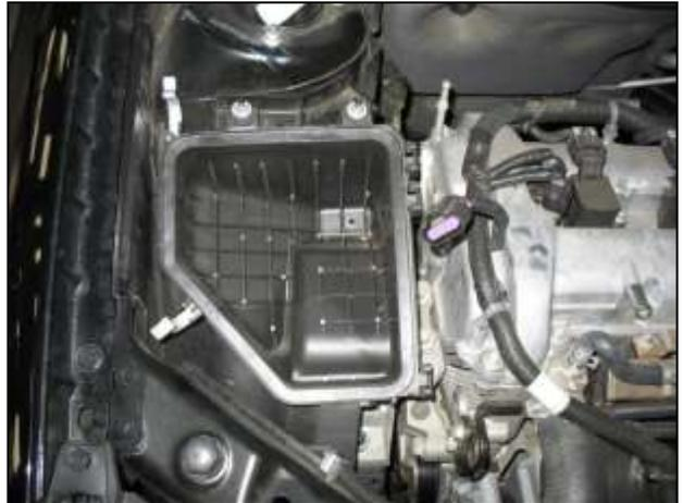
h. Pull straight up on the factory air lid assembly and remove it from the vehicle. Also, remove the stock air filter. Then remove the two nuts securing the lower air filter assembly in place and remove it from the vehicle.
