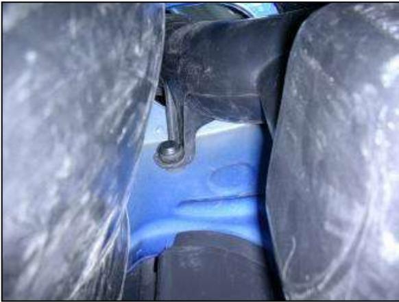
i. Remove the front passenger side fender liner to gain access to the lower air box. From inside the fender, release the plastic retainer near the top of the lower air box.
