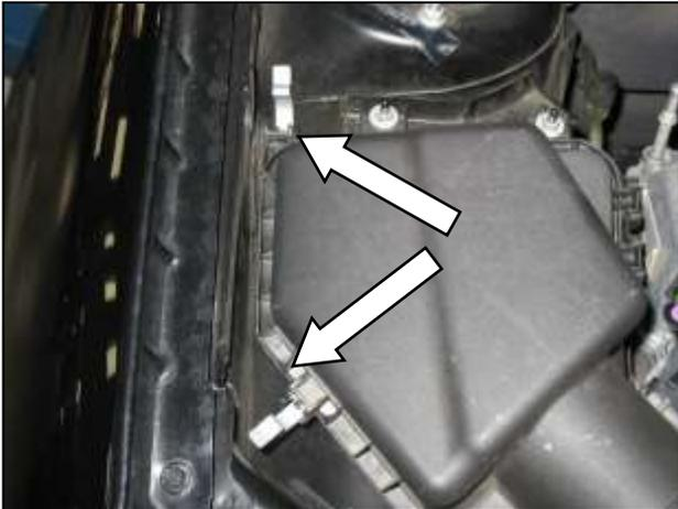
g. Release the two clips holding the air filter lid in place.
