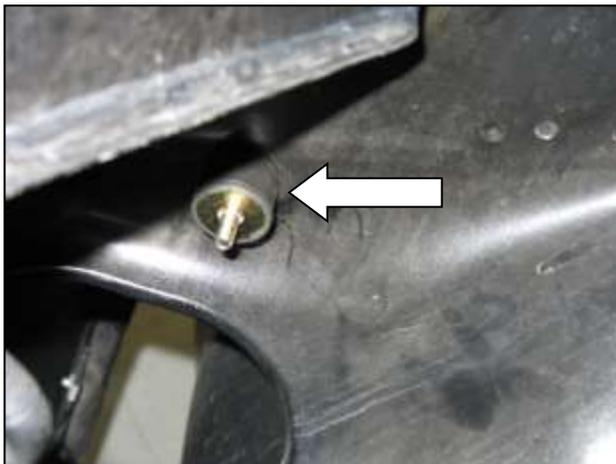
b. Install the supplied rubber mount into the hole where the factory lower air box was located.
