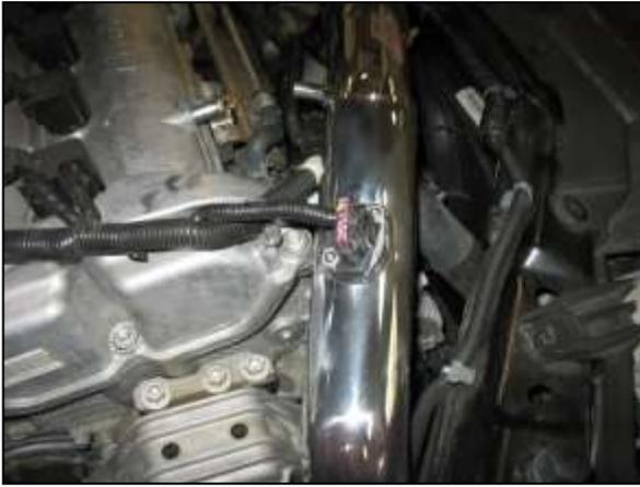
g. Use supplied bolts to secure the MAF sensor to the intake pipe. Then connect the wiring harness to the sensor.
