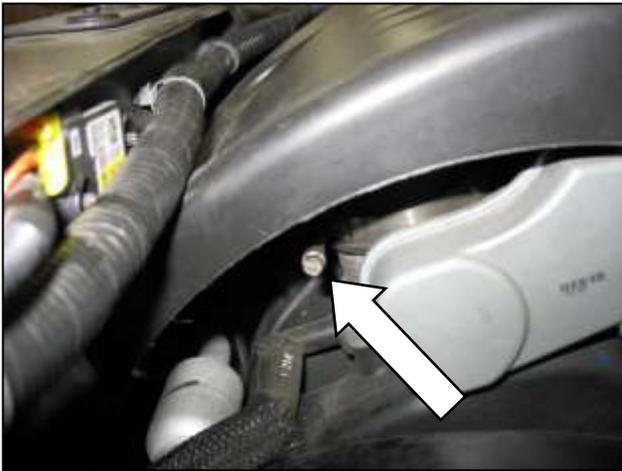
e. Loosen the hose clamp securing the stock inlet tube to the throttle body.
