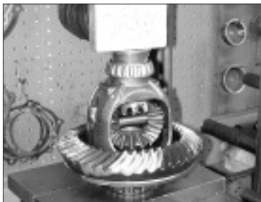
Pressing on carrier bearing
