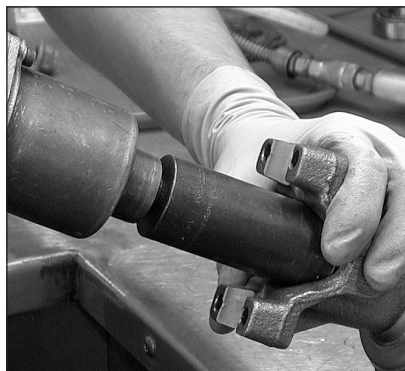
1/2" impact gun on pinion nut
