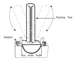
**ROPE SEALS:** Install the seals into the grooves of the cap and block by firmly pressing the packing into the grooves using a "packing tool".
