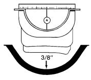
Use %" (thick) seal on oil pans having "A" dimension of 2%"
